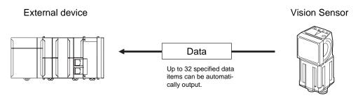
You must specify in advance the data to output (up to 32 items) after measurements. That data is sent to the external device in either ASCII or binary format through a continuous serial connection. There is no handshaking from the external device to confirm if it can receive the data.
