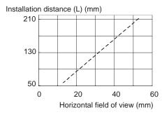
The optical chart indicates the horizontal field of view. The vertical field of view depends on the model as follows: FQ2-CH
