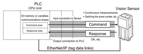
To send a control command, you write a control command to the command area (i.e., a variable or I/O memory address in the PLC) that is specified for the output tag, and then turn ON the Command Execution (EXE) Bit. As a result, the control command is sent through the input connection from the PLC to the Vision Sensor.
