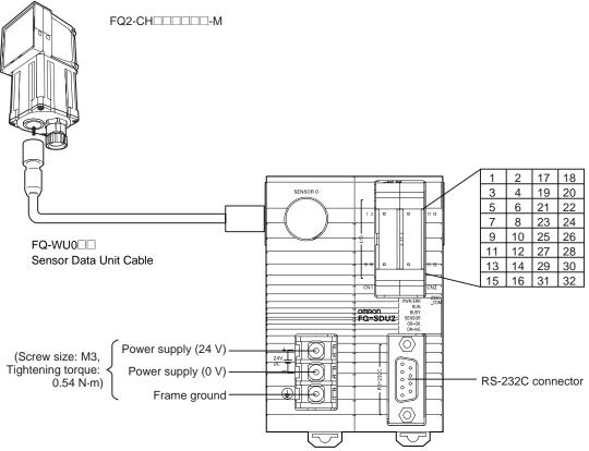
For the I/O connector harness, use an FQ-VP2 Parallel Cable for the FQ-SDU2 or a MIL-standard harness, such as the OMRON XZ2F. (The Cables are sold separately.)
