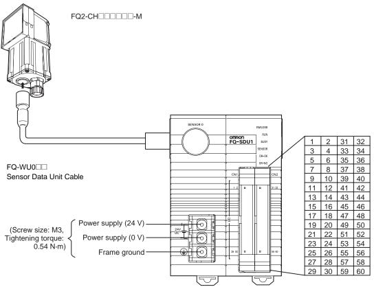
For the I/O connector harness, use an FQ-VP1 Parallel Cable for the FQ-SDU1 or a MIL-standard harness, such as the OMRON XZ2F. (The Cables are sold separately.)
