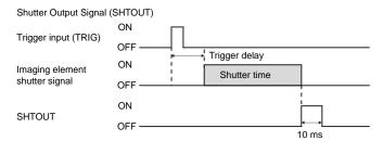
The SHTOUT signal turns ON for approximately 10 ms (fixed) when the shutter time (exposure period) elapses after the trigger is input from an external device.
