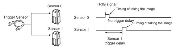
Sensor 0 immediately begins image input when the trigger is input. Sensor 1 begins image input after the specified time has passed.
