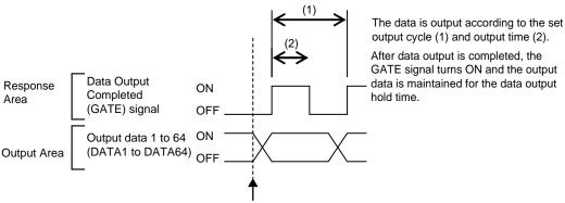
Here, the Vision Sensor ends measurements and can output data.
