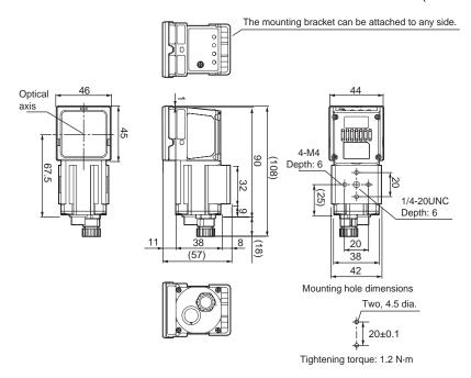
FQ2-CH10100F-M/-CH10100N-M FQ2-CH15100F-M/-CH15100N-M (Unit: mm)
