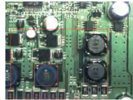
Second inspection: Checking for Presence of Electronic Components on the PCB
