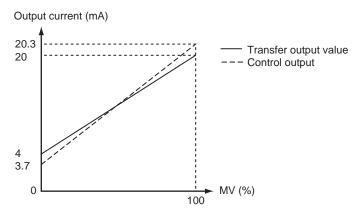
(The above graph is for when the linear current output type is set to 4 to 20 mA.)
