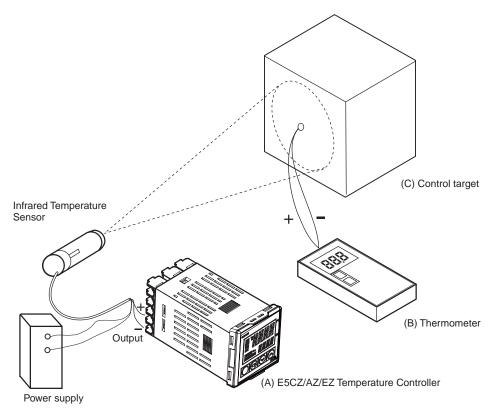
Figure 1 Offset Configuration for an Infrared Temperature Sensor
