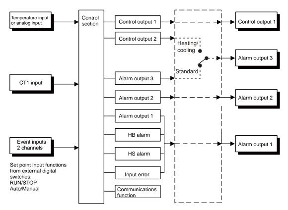
**Note** Functions can be assigned individually for each output by changing the set values for the control output 1 assignment, the alarm output 1 assignment, the
