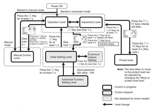
**Note** (1) Moves to operation level by software reset.
