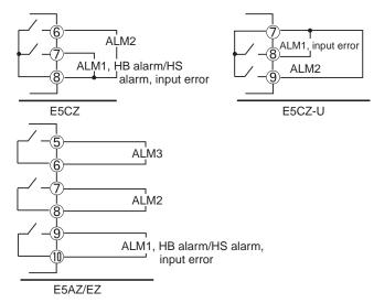
ALM 1, 2, 3 can be output to alarm output 1, 2, 3, or changed with the advanced function setting level.
