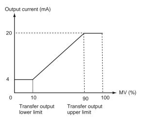
(The above graph is for when the linear current output type is set to 4 to 20 mA.)
