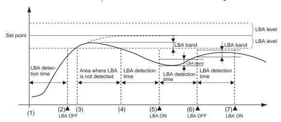
If the control deviation is reduced in the area between 1 and 2 (i.e., the set point is approached) and the amount the control deviation is reduced is at least equal to the LBA band, the loop break alarm will remain OFF.
