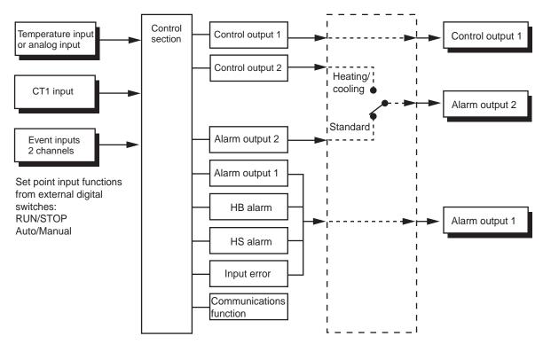
**Note** Functions can be assigned individually for each output by changing the set values for the control output 1 assignment, the alarm output 1 assignment, and the alarm output 2 assignment in the advanced function setting level.
