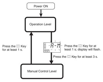
To move from the operation level to the manual control level, press the O key for at least three seconds with the "auto/manual switch" parameter displayed.
