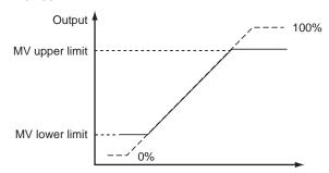
• For heating/cooling control, upper and lower limits are set of overall heating/cooling control. (They cannot be set separately for heating/cooling.)
