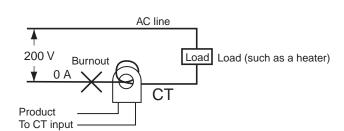
The heater power supply provides 5 A when the current is normal, and 0 A when there is a burnout, so the heater burnout detection current is calculated as follows:
