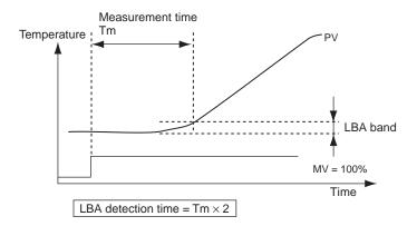
Loop Break Alarm Section 4-11
