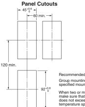
Recommended panel thickness is 1 to 8 mm. Group mounting is not possible. (Maintain the specified mounting space between Controllers.)
