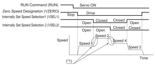
\*1. The acceleration time, deceleration time, and S-curve acceleration/deceleration time can be set using parameters (Pn58, Pn59, and Pn5A).
