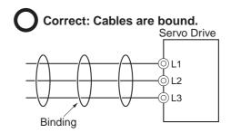
· Separate power supply cables and signal cables when wiring.
