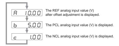
Note: The displayed value will not be accurate if the voltage exceeds ±10 V.
