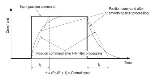
• If the setting is 0, the control cycle will be  $(0 + 1) \times 166 = 166 \,\mu s$ . If the setting is 1, the control cycle will be  $(1 + 1) \times 166 = 332 \,\mu s$ . Likewise, if the setting is 31, the control cycle will be  $(31 + 1) \times 166 = 5,312 \,\mu s$ .
