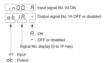
• Displays the status of the control input and output signals connected to CN1.
