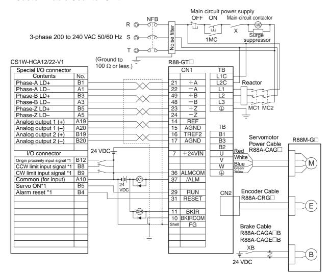
\*1. The I/O bits for the CS1W-HCA12/22 depend on the memory allocations in the CIO Area. Change the wiring according to the allocations.
