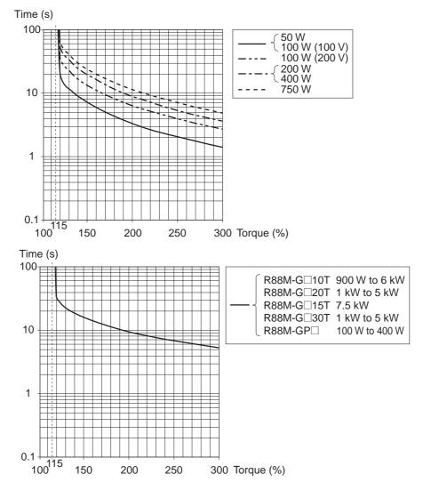
When the torque command = 0, and a constant torque command is continuously applied after three or more times the overload time constant has elapsed, the overload time t [s] will be: t [s] = - Overload time constant [s]  $\times$  log<sub>e</sub> (1 - Overload level [%] / Torque command [%])  $^2$
