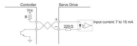
• Select a resistance R value so that the input current will be from 7 to 15 mA. Refer to the following table.
