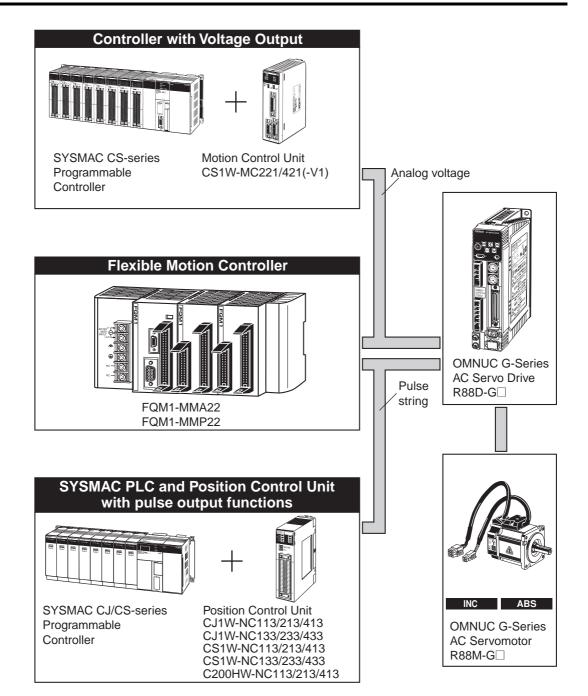
Servomotors with absolute encoders can be used in combination with CS1W-MC221/421(-V1)
