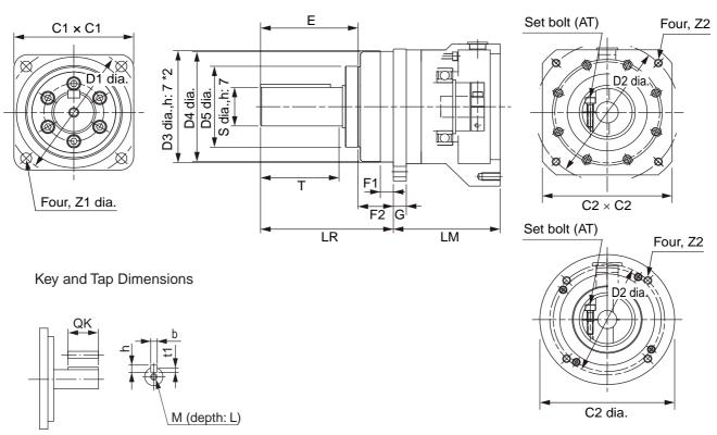
\*2. With the R88G-HPG50 $\square$ , the height tolerance is 8 mm (D3 dia., h: 8).
