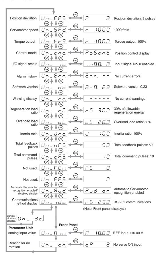
• The Servomotor speed will be displayed the first time the power is turned ON after purchase. To change the initial display when the power is turned ON, change the setting for the Default Display (Pn01). For details, refer to *Pn01 Default Display* on page 5-52.
