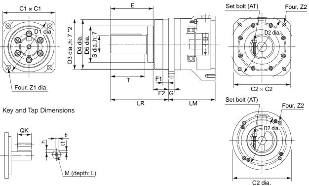
\*2. With the R88G-HPG50 $\square$ /-HPG65 $\square$ , the height tolerance is 8 mm (D3 dia., h: 8).
