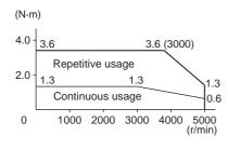
3,000-r/min Servomotors with 200-VAC Power Input
