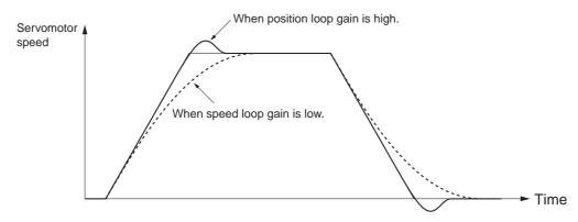
• If the speed loop gain and position loop gain are optimally set, the Servomotor operation for the command will be delayed 2/Kp at acceleration and delayed 3/Kp at deceleration.
