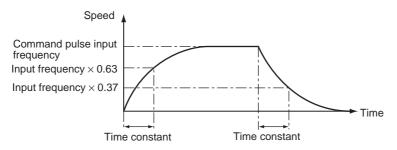
**Note** The time constant will be as follows according to the setting of Pn4C.
