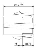
Connector housing: 172160-1 (Tyco Electronics AMP KK) Contact socket: 170365-1 (Tyco Electronics AMP KK)
