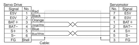
3 to 20 m: Crimp-type I/O Connector (Molex Japan) 30 to 50 m: 55100-0670 (Molex Japan)
