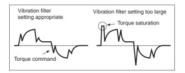
The vibration filter setting is restricted by the following equation.
