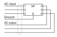
• Use twisted-pair cables for the power supply cables, or bind the cables.
