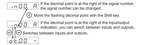
The following procedure can also be used to switch between inputs and outputs.
