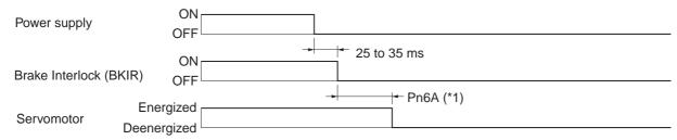
\*1. The time from turning OFF the brake power supply to the brake engaging is 100 ms max. If using the Servomotor on a vertical axis, take this delay into account and set the Brake Timing when Stopped (Pn6A) so that the Servomotor is deenergized after the brake has engaged.
