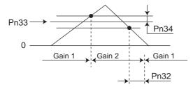
• The settings for the Gain Switch 1 Level Setting (Pn33) and the Gain Switch 1 Hysteresis Setting (Pn34) are effective as absolute values (positive/negative).
