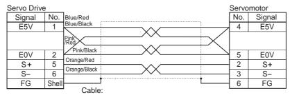
Servo Drive Connector AWG24×4P UL20276
