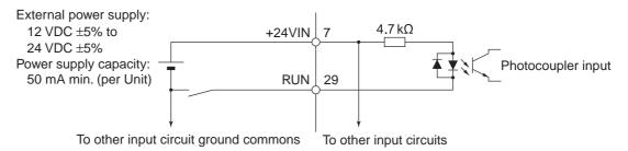
Signal Levels ON level: 10 V min. OFF level: 3 V max.
