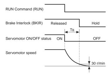
"TB" in the above figure is the brake timing during operation (setting  $\times$  2 ms) or the time until the speed of the Servomotor falls to 30 r/min or lower, whichever is shorter.
