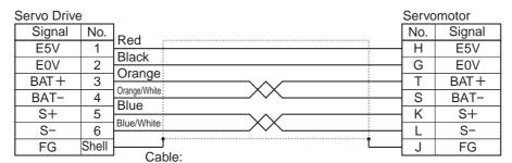
Servo Drive Connector AWG22 x 2C + AWG24x2P UL20276 (3 to 20 m) AWG16 x 2C + AWG26x2P UL20276 (30 to 50 m)
