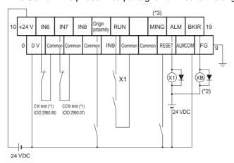
\*1. CW and CCW limit input signals can also be input through Input Units. The bits for the CW/CCW limit inputs in the CJ1M are as follows: CW: A540.08, CCW: A540.09 for pulse output 0 and CW: A541.08, CCW: A541.09 for pulse output 1. For example, the flag for the CW limit input (A540.08) can be controlled with an output from the ladder diagram using a bit allocated to the actual input (CIO 2960.06) on the Input Unit, as shown below.
