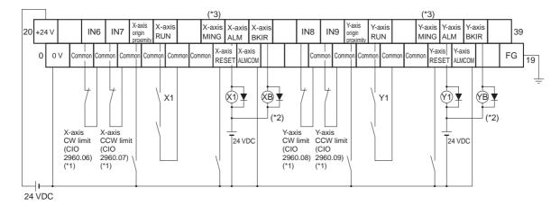
\*1. CW and CCW limit input signals can also be input through Input Units. The bits for the CW/CCW limit inputs in the CJ1M are as follows: CW: A540.08, CCW: A540.09 for pulse output 0 and CW: A541.08, CCW: A541.09 for pulse output 1. For example, the flag for the CW limit input (A540.08) can be controlled with an output from the ladder diagram using a bit allocated to the actual input (CIO 2960.06) on the Input Unit, as shown below.
