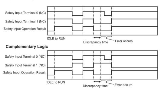
Emergency Stop Switches, Door Switches, Limit Switches, Light Curtains, Other Input Devices (Single Channel Inputs), Reset Switches, and Welding Check (EDM) Feedback Inputs
