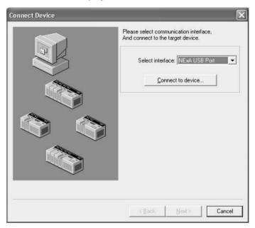
3. Select an interface for connecting to the network and click the **Connect to device** Button. Click the **Refresh** Button when the window to search for the destination device is displayed.
