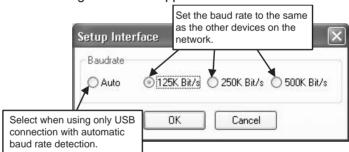
**IMPORTANT** If there are other devices already online on the same network, set the baud rate to the same baud rate as the devices. If devices on the network have different baud rates, a bus off error will occur, and communications will not function correctly.
