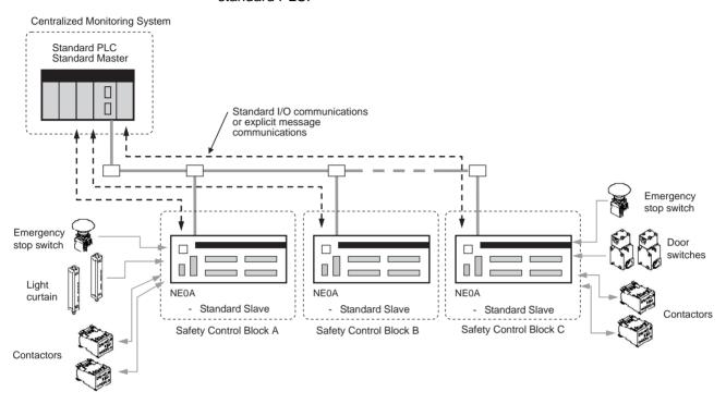
**IMPORTANT** The data attributes handled by standard I/O communications and explicit message communications are non-safety data. The necessary measures for safety data are not taken for this data during data generation. Therefore, do not use this data to configure the Safety Control System.
