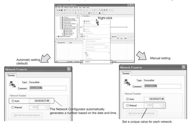
**IMPORTANT** Set a unique network number for each network. If connections are made to more than one network with the same network number, the system may operate unpredictably.
