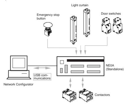
**IMPORTANT** Use a USB port connection to set Standalone Mode. DeviceNet communications are stopped when Standalone Mode is set, and so setting is not possible from the DeviceNet port.
