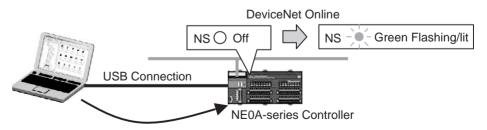
Connected online to DeviceNet at the specified baud rate.
