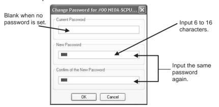
**Note** For details on device passwords, refer to the *DeviceNet Safety System Configuration Manual* (Cat. No. Z905).
