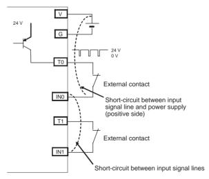
If an error is detected, safety input data and individual safety input status will turn OFF.
