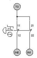
If detecting short-circuits between input wiring is not required.
