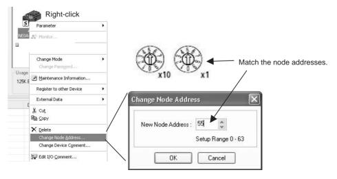
**Note** The node addresses will affect memory allocations of the I/O Memory Area for the OMRON CS/CJ-series DeviceNet Master Unit if fixed allocations are used
