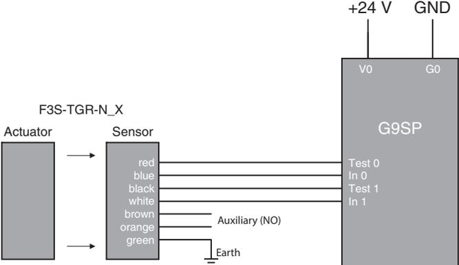
Series connection Application, up to 6 Sensors with G9SP
