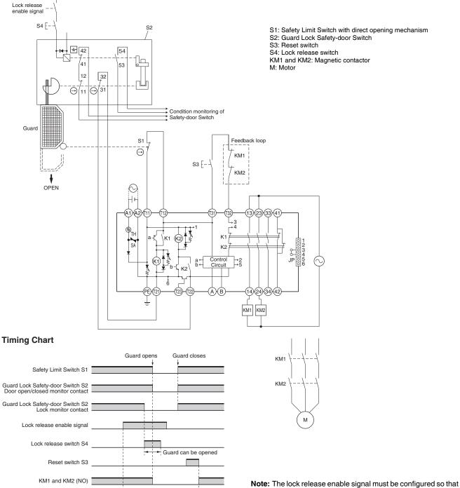
it should turn ON after dangerous movement is stopped and safety is ensured for the door to open.
