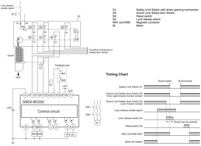
**Note:** The lock release enable signal must be configured so that it should turn ON after dangerous movement is stopped and safety is ensured for the door to open.
