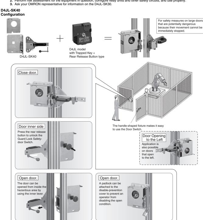
Note: This example shows a D4JL Switch with a trapped key and rear release button (D4JL-\\_\\_\\_\-\\_\-\\_\-\\_\-SJ).
