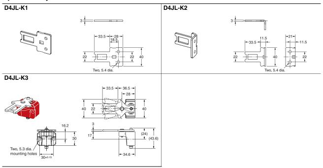
Note: Unless otherwise specified, a tolerance of ±0.8 mm applies to all Switch dimensions and a tolerance of ±0.4 mm applies to Operation Key dimensions.
