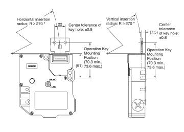
D4JL + D4JL-K2 (with Front-inserted Operation Key)
