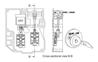
(5) Operation Key inserted, solenoid ON, and trapped key removed. Status: Door unlocked.
