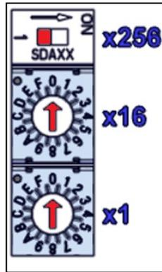
Figure 3-8. EtherCAT Node ID 0 Switch Setting
