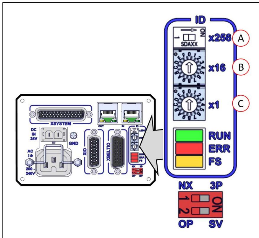
Figure 3-9. Robot Interface Panel EtherCAT ID Switches
