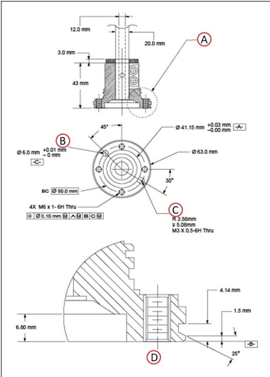
Figure 8-20. Tool Flange Dimensions for eCobra Robots
