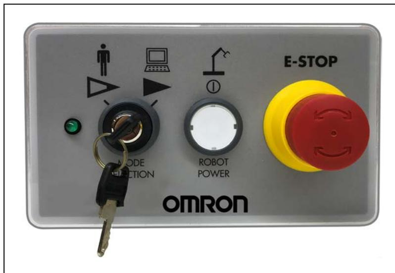
Figure 6-8. Front Panel Keyswitch in Auto
