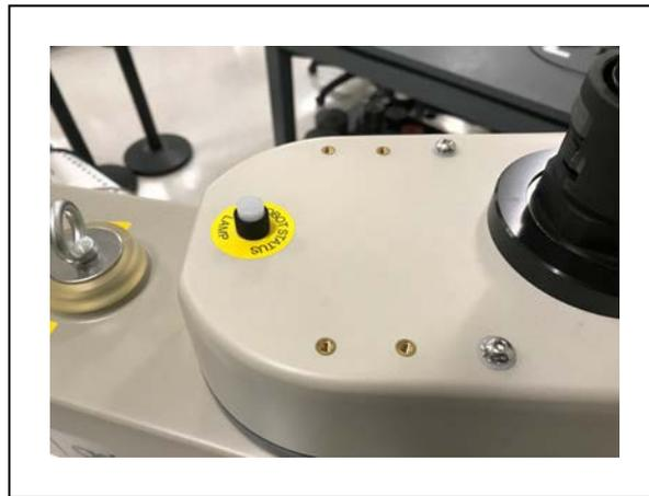
Figure 5-2. External Equipment Mounting location, J1
