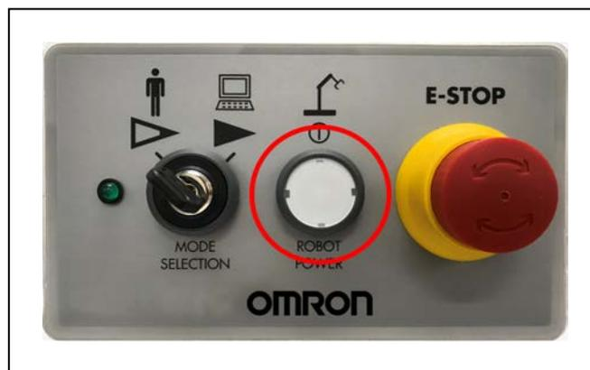
Figure 6-6. High Power Button on Front Panel
