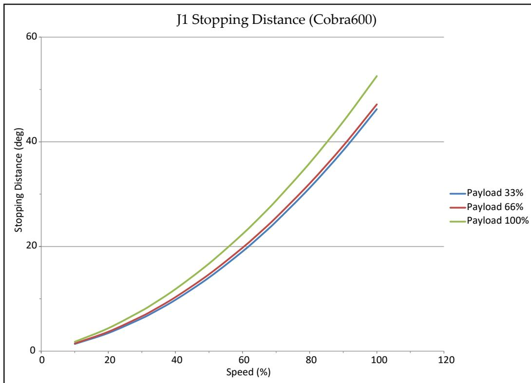
Figure 8-8. Stopping Distance in Degrees versus Speed % for eCobra 600, Joint 1
