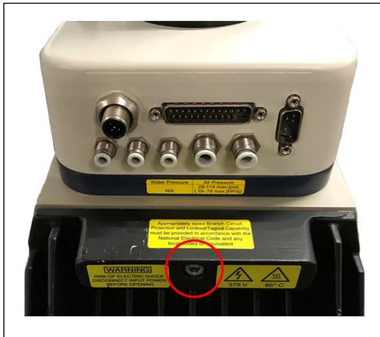
Figure 7-9. Securing Screw on iCS-ECAT Chassis
