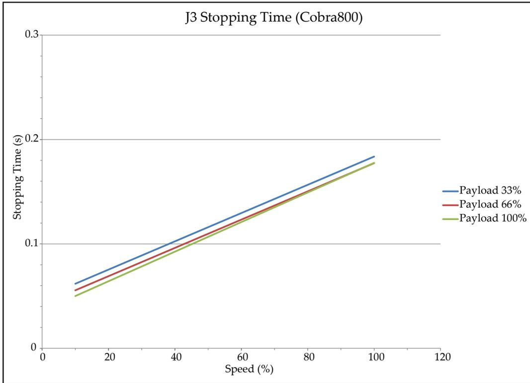
Figure 8-19. Stopping Time in Seconds versus Speed (%) for eCobra 800, Joint 3
