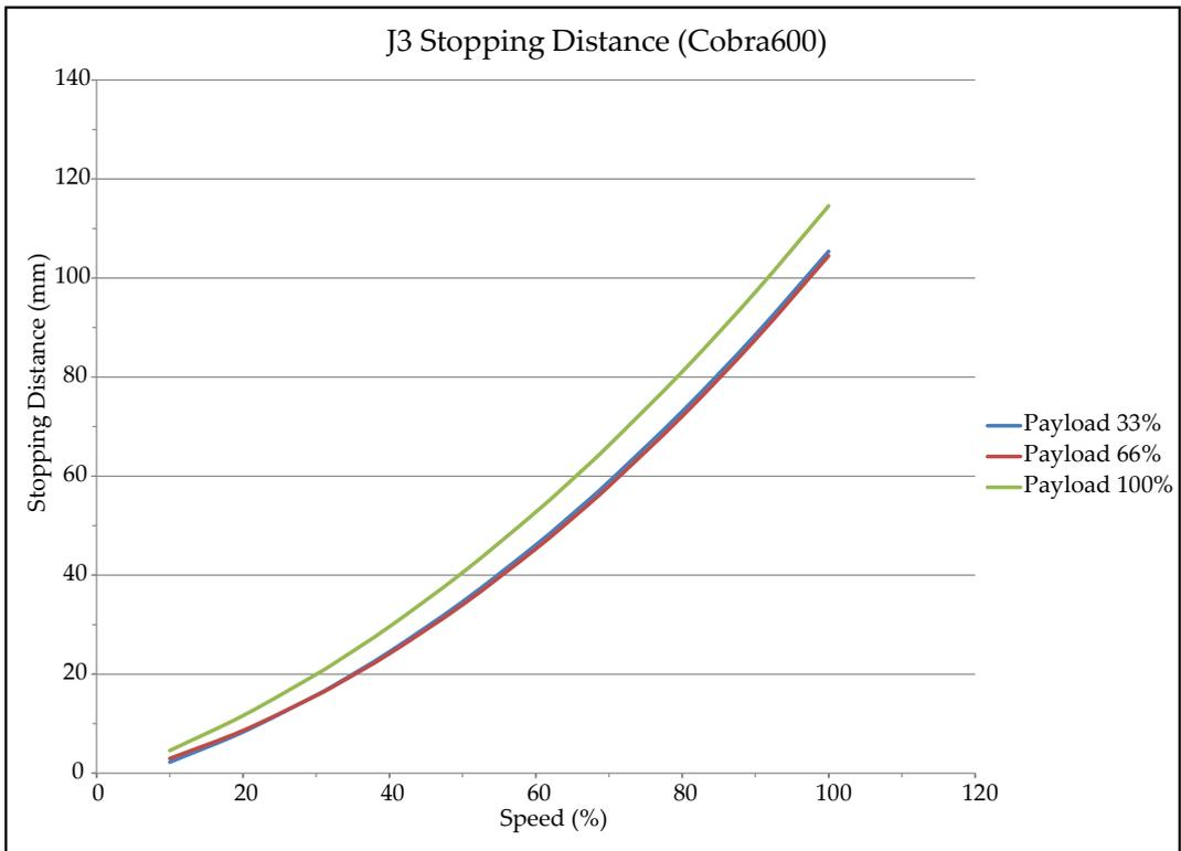
Figure 8-12. Stopping Distance (mm) versus Speed (%) for eCobra 600, Joint 3
