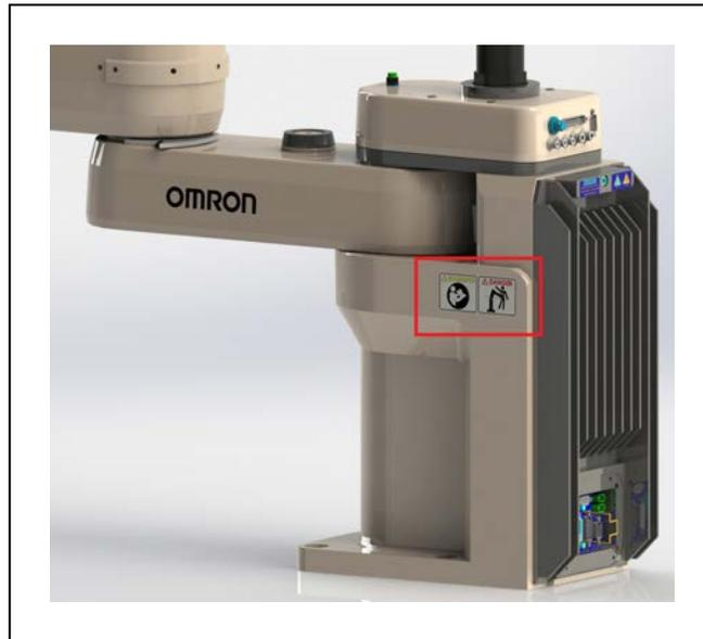
Figure 7-2. Location of Read Manual and Impact Warning Label
