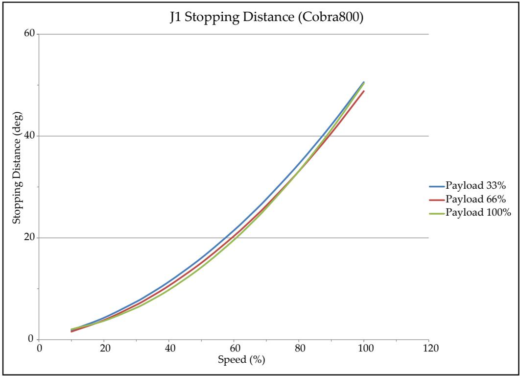
Figure 8-14. Stopping Distance in Degrees versus Speed (%) for eCobra 800, Joint 1
