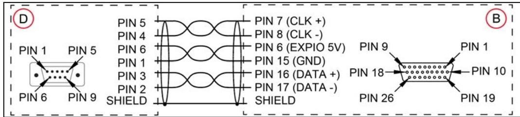
Figure 4-5. XBELT I/O Adapter Cable Pinout - EXPIO Connections
