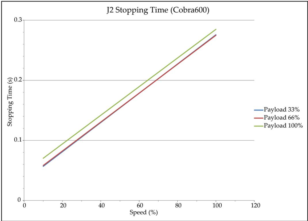
Figure 8-11. Stopping Time in seconds versus Speed % for eCobra 600, Joint 2
