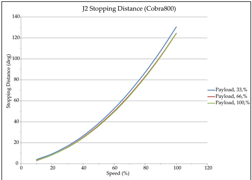
Figure 8-16. Stopping Distance in Degrees versus Speed (%) for eCobra 800, Joint 2
