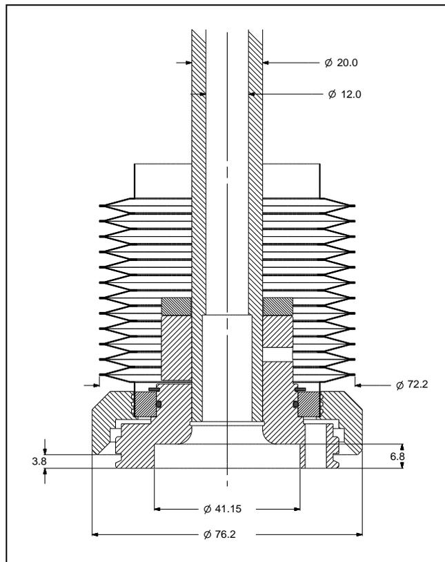
Figure 9-2. eCobra 800 IP65 Tool Flange (units in mm)
