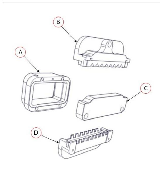
Figure 9-4. Cable Seal Parts Assembly
