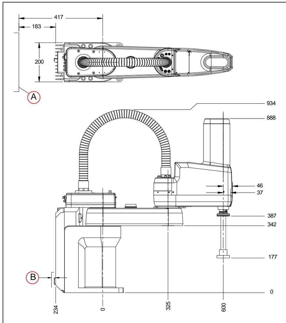
Figure 8-1. eCobra 600 robot Top and Side Dimensions (units in mm) where (A) is the (required clearance to open iCS-ECAT chassis, and (B) is the required cable clearance of 31 mm
