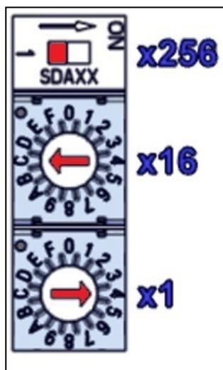
Figure 3-10. EtherCAT Node ID Set to 196
