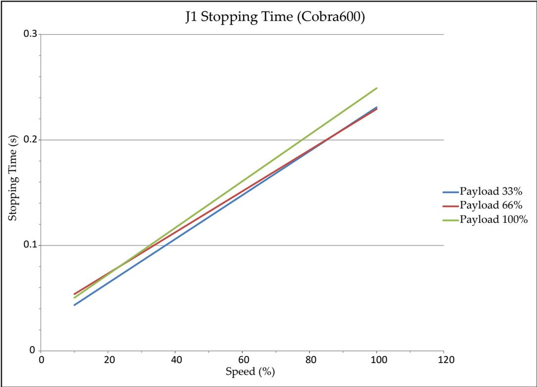
Figure 8-9. Stopping Time in Seconds versus Speed% for eCobra 600, Joint 1
