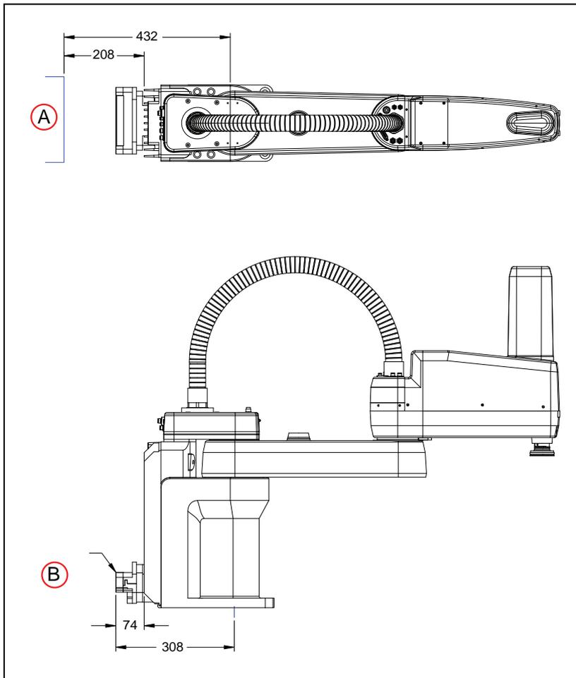
Figure 9-9. Cable Seal Assembly Dimensions showing required clearance to open iCS-ECAT controller with IP65 connector (A), and dimensions of cable sealing box on IP65 version (B) (units in mm)
