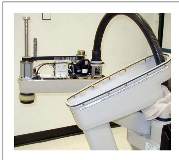
Figure 9-11. IP65 Robot with Outer Link Cover Removed
