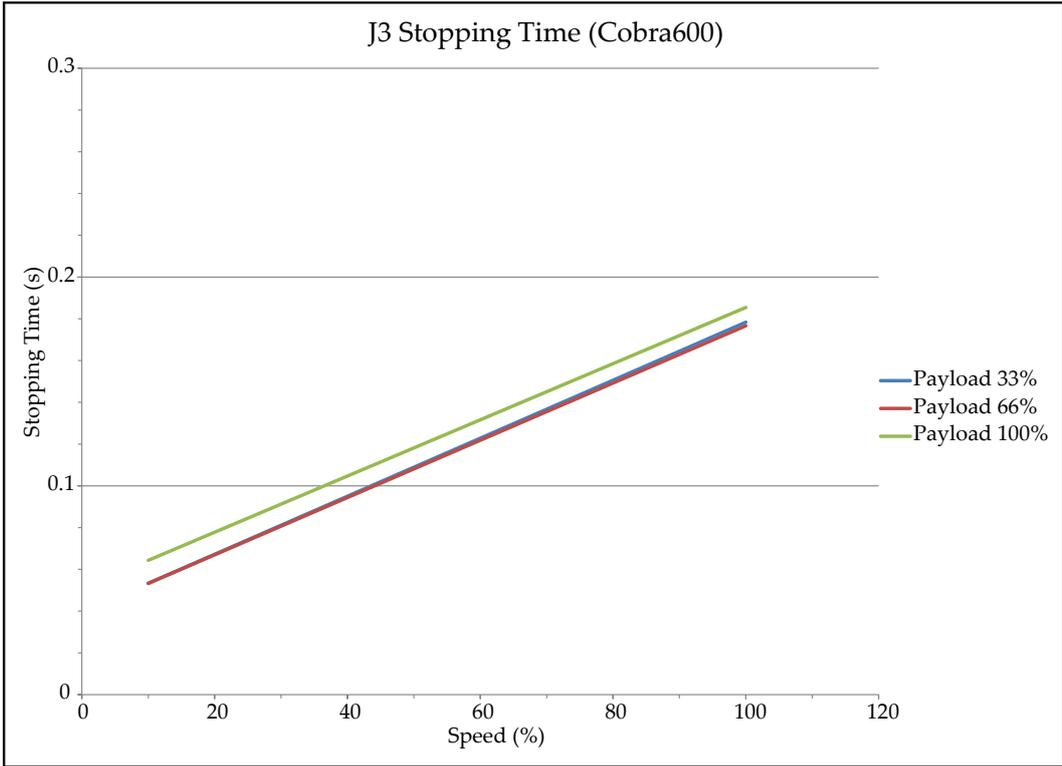
Figure 8-13. Stopping Time in Seconds versus Speed (%) for eCobra 600, Joint 3
