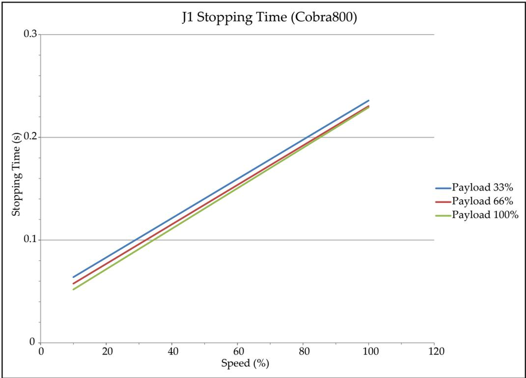
Figure 8-15. Stopping Time in Seconds versus Speed (%) for eCobra 800, Joint 1
