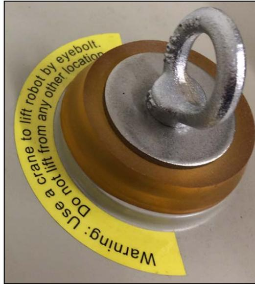
Figure 7-4. Lifting Eyebolt Label
