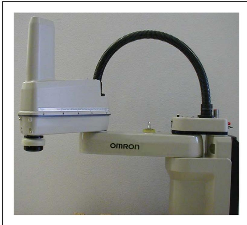
*Figure 9-1. eCobra 800 Robot—IP65 Option*
