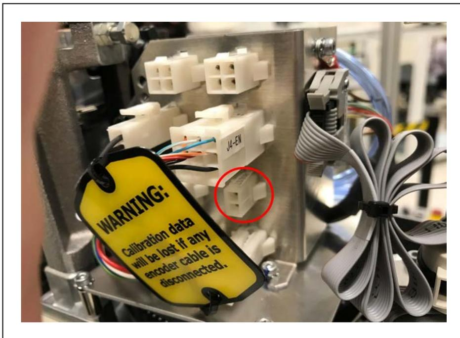
Figure 1-12. End of Arm Break-away Sensor Connector Location
