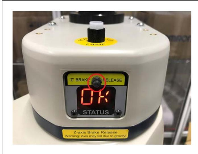
Figure 6-4. Brake Release Button
