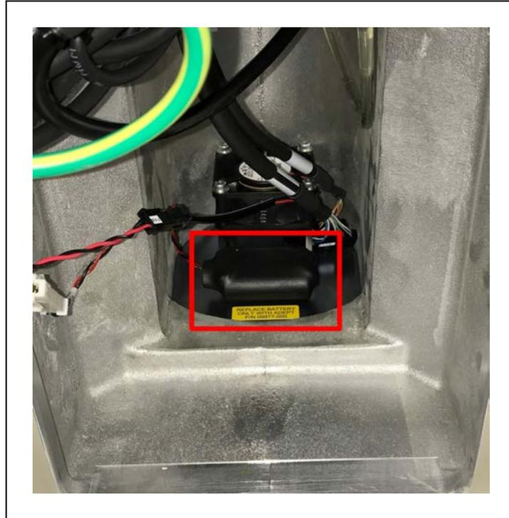
Figure 7-7. Location of Encoder Battery Pack in the robot base interior
