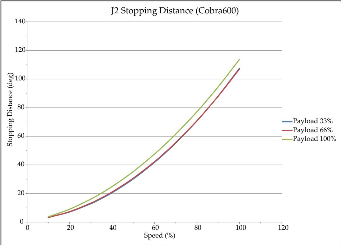
Figure 8-10. Stopping Distance in Degrees versus Speed % for eCobra 600, Joint 2
