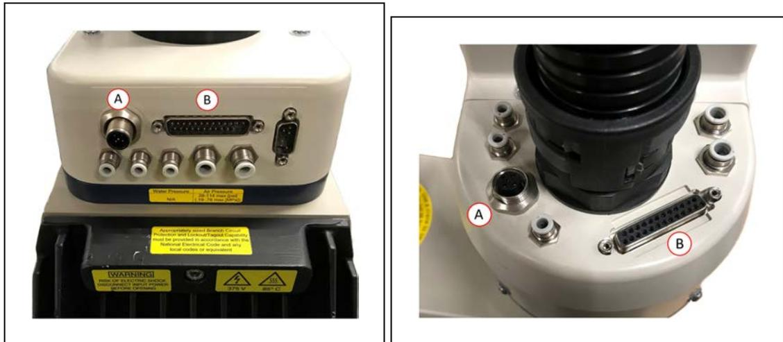
Figure 1-8. User Electrical Connectors on Joint 1 (left) and Joint 2 (right)
