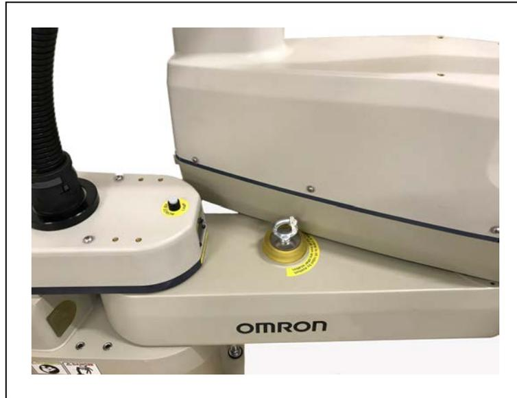
Figure 3-2. Lifting Eye Bolt
