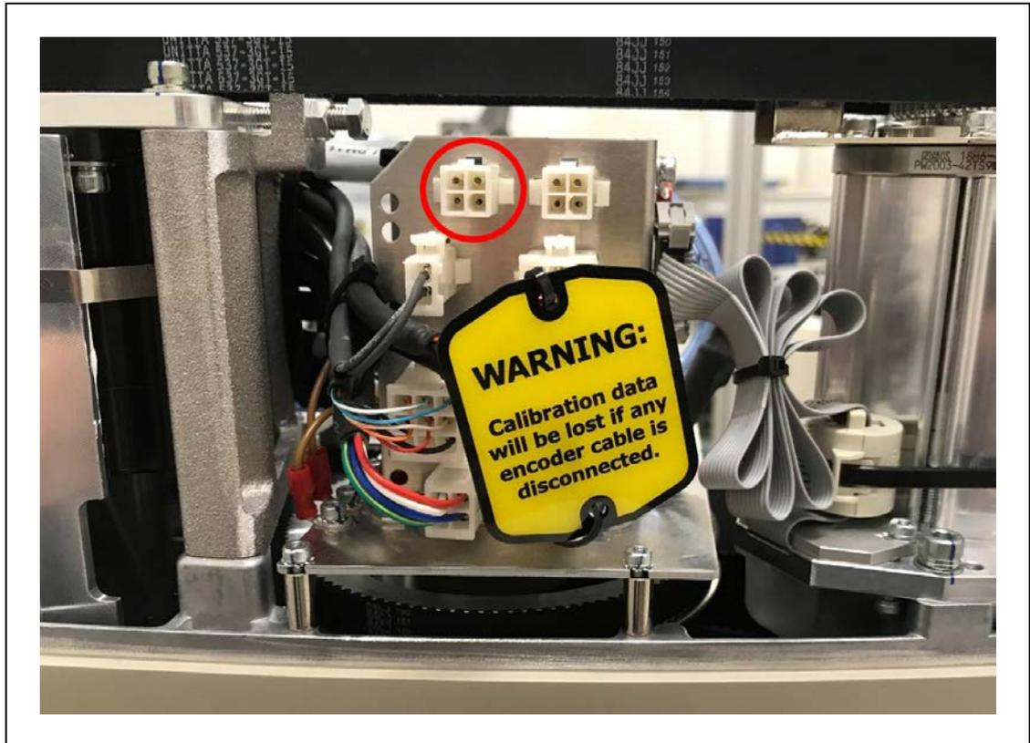
Figure 1-11. OP3/4 Connector Location
