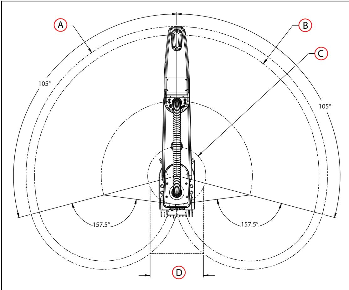
Figure 8-7. eCobra 800 Robot Working Envelope
