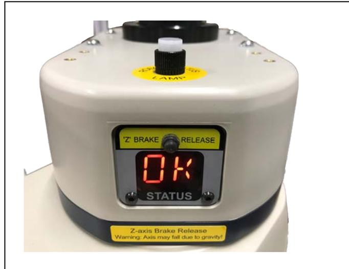
Figure 6-7. Robot Status Display and LED
