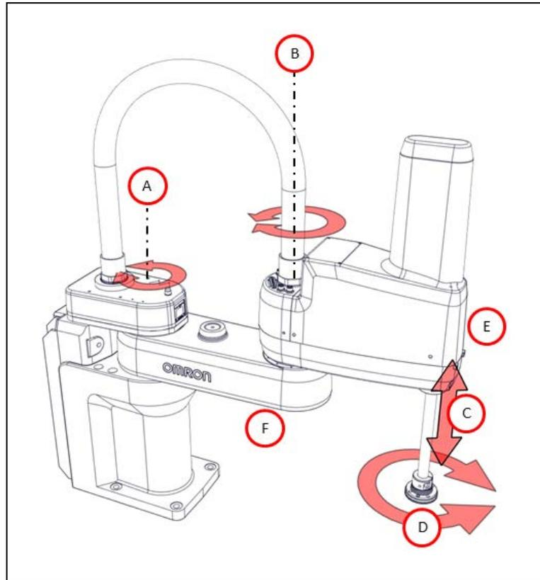
Figure 1-6. Robot Joint Motions - eCobra 600 Robot Shown
