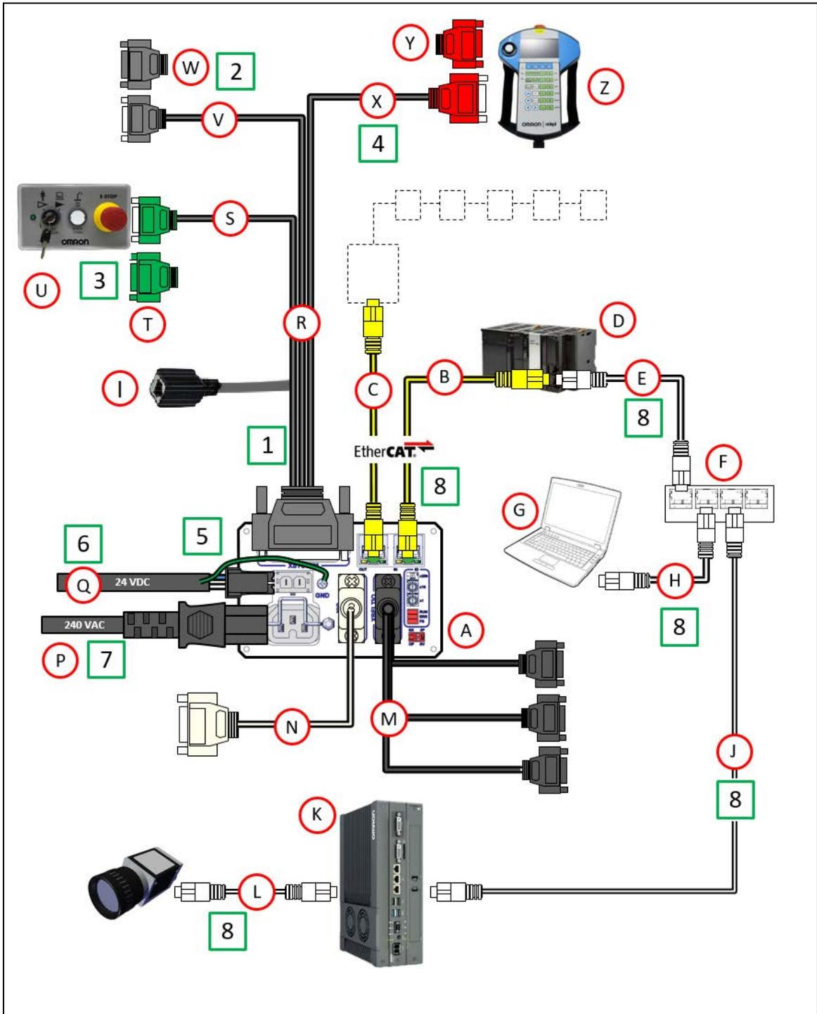
Figure 4-1. Typical System Cable Connections
