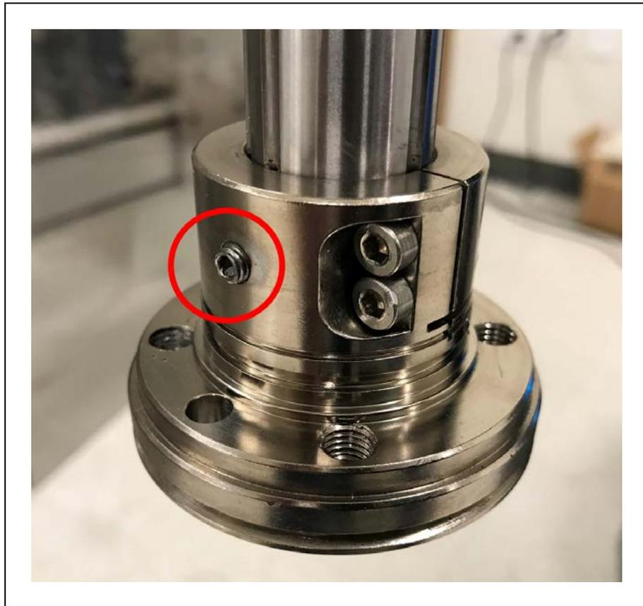
Figure 7-8. Tool Flange Setscrew
