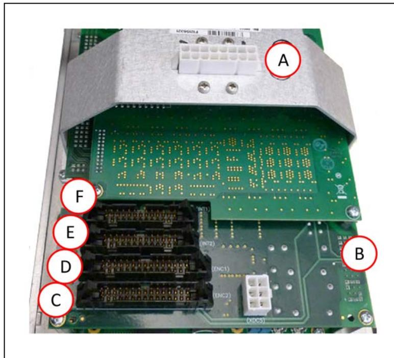
Figure 7-11. Connectors on Chassis and ePMAI Board
