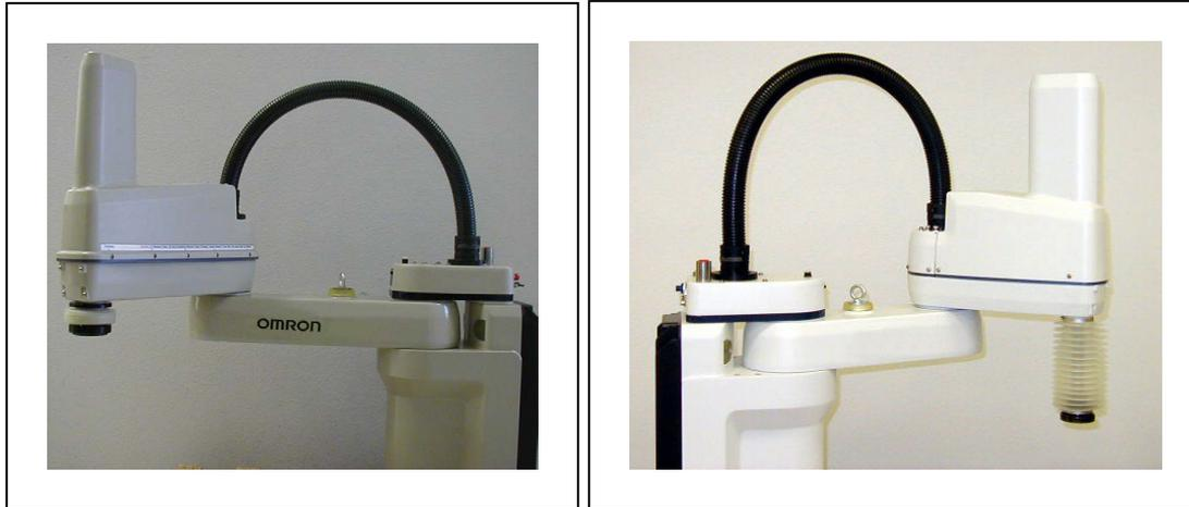
Figure 1-5. IP65 Version (left), Cleanroom Version (right)
