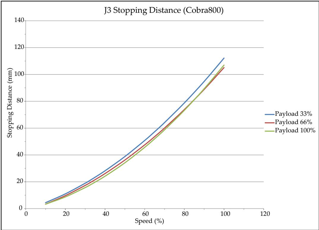
Figure 8-18. Stopping Distance in Millimeters versus Speed (%) for eCobra 800, Joint 3
