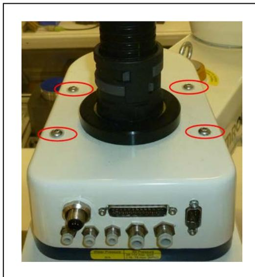
Figure 5-10. Joint 1 Cover Screws (circled)
