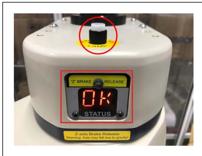
Figure 6-2. Robot Status LED and Display Panel
