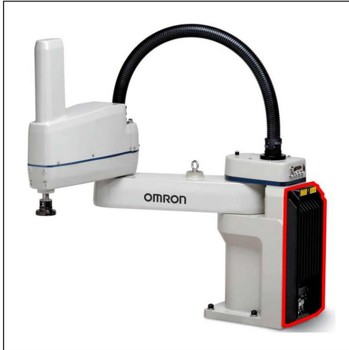
*Figure 1-3. eCobra Robot with iCS-ECAT Highlighted*
