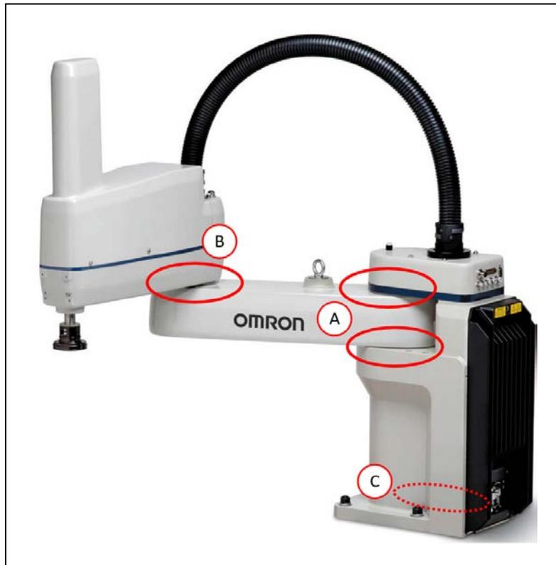
Figure 7-5. eCobra Oil Leak Inspection Areas
