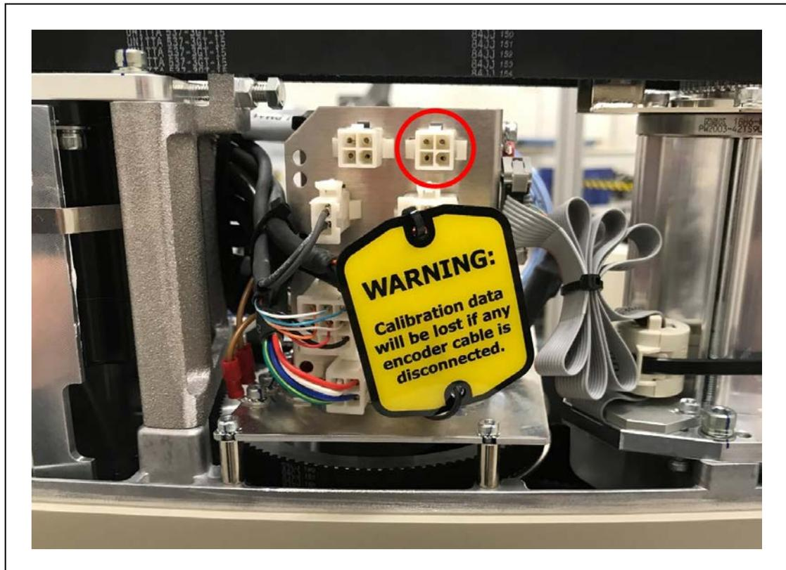
Figure 1-13. EOAPWR Connector Location
