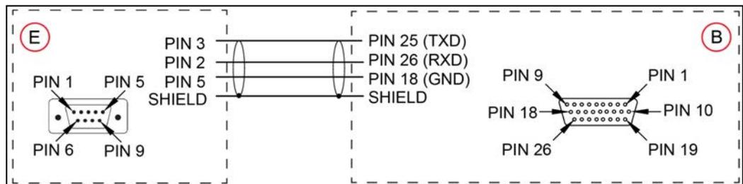
Figure 4-4. XBELT I/O Adapter Cable Pinout - RS-232 Connections
