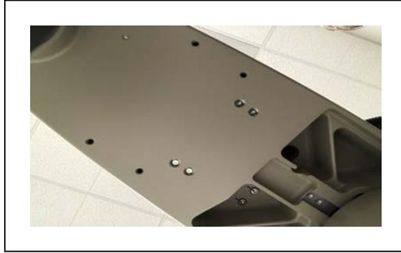
Figure 5-4. External Tooling Location, Outer Link (bottom)
