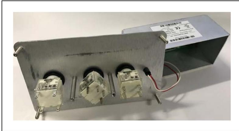
*Figure 7-16. Removing Robot Power Lamp (twisted center lamp)*
