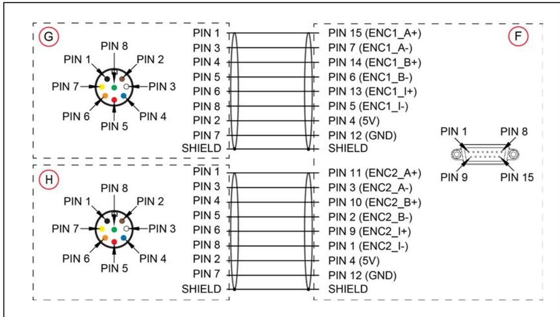
Figure 4-6. Belt Y Splitter Cable Pinout - 2 Encoder Connections
