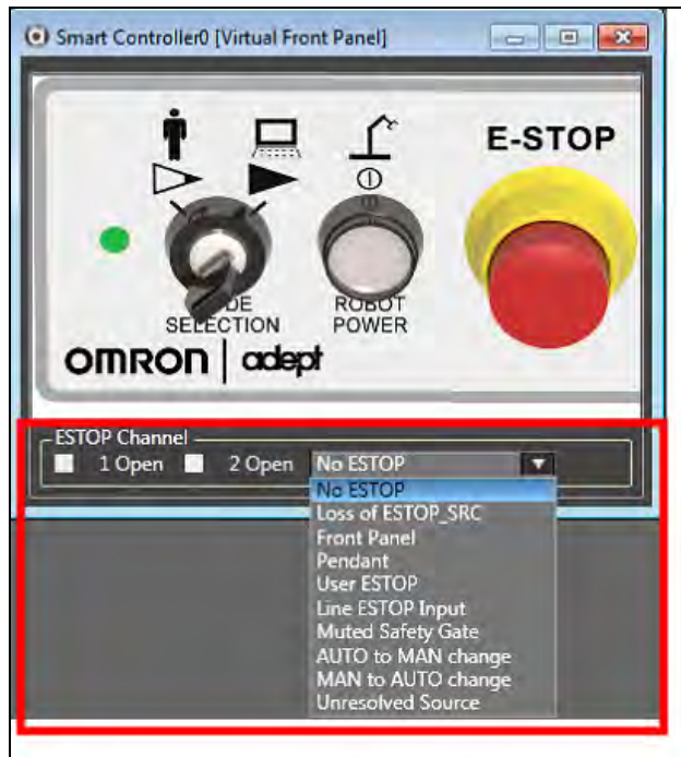
Figure 5-49 E-STOP Channel Simulation Functions
