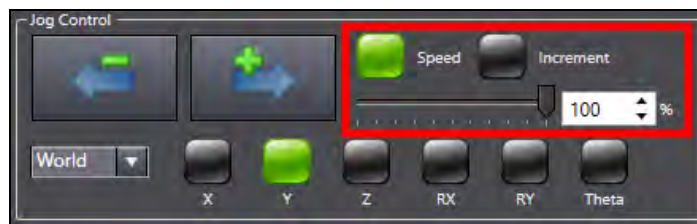
Figure 5-35 V+ Jog Control - Speed, Increment Selection Buttons
