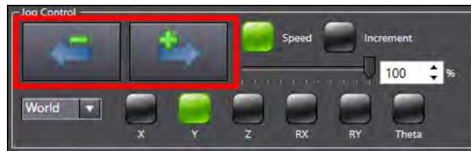
Figure 5-34 V+ Jog Control - Move Axis Buttons
