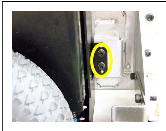
Figure 8-16. Mounting Screws at Bottom-Right of Drive Assembly
