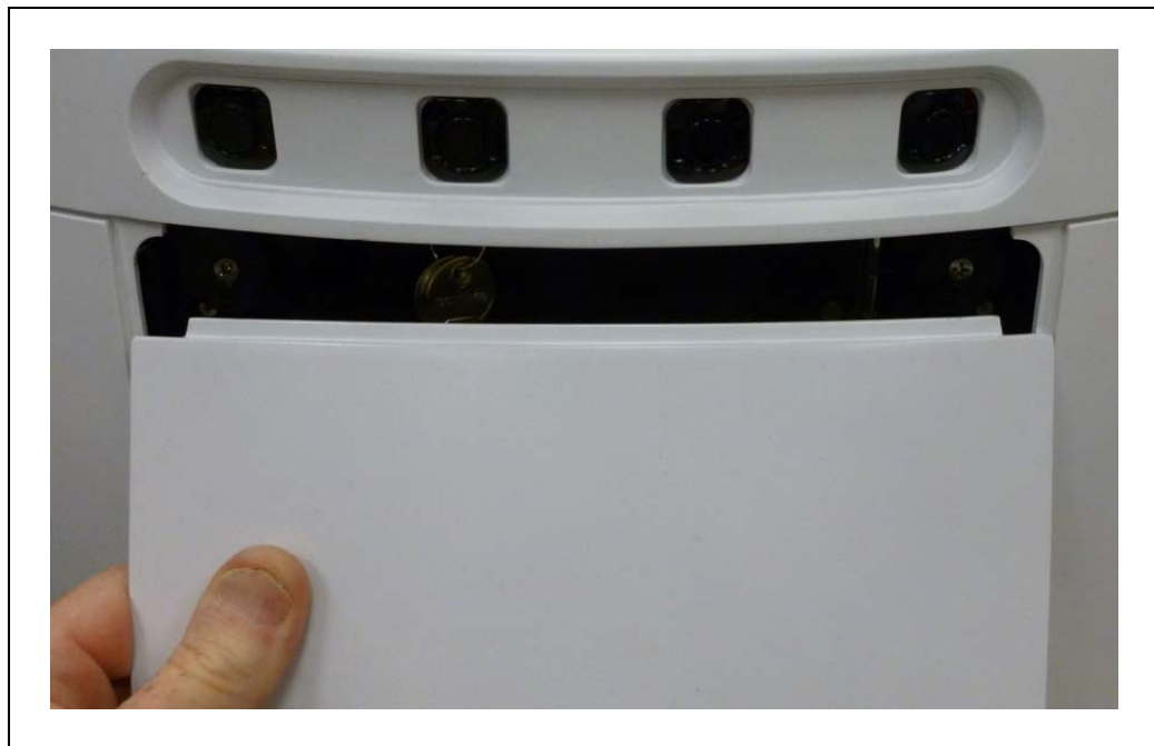
Figure 3-15. Lowering the Battery Door Platform Skin
