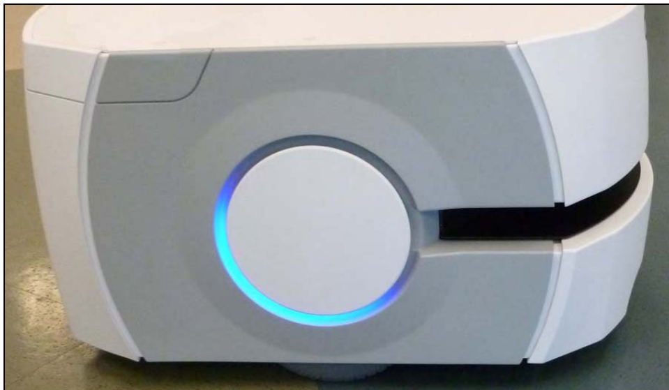
Figure 8-22. Right Side Skin, Showing Even Gaps at Edges
