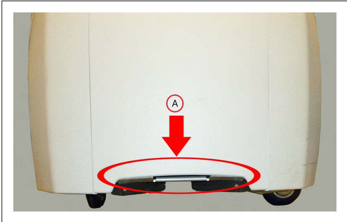
Figure 8-3. Bottom of Battery Door Skin. (A) Lift Here
