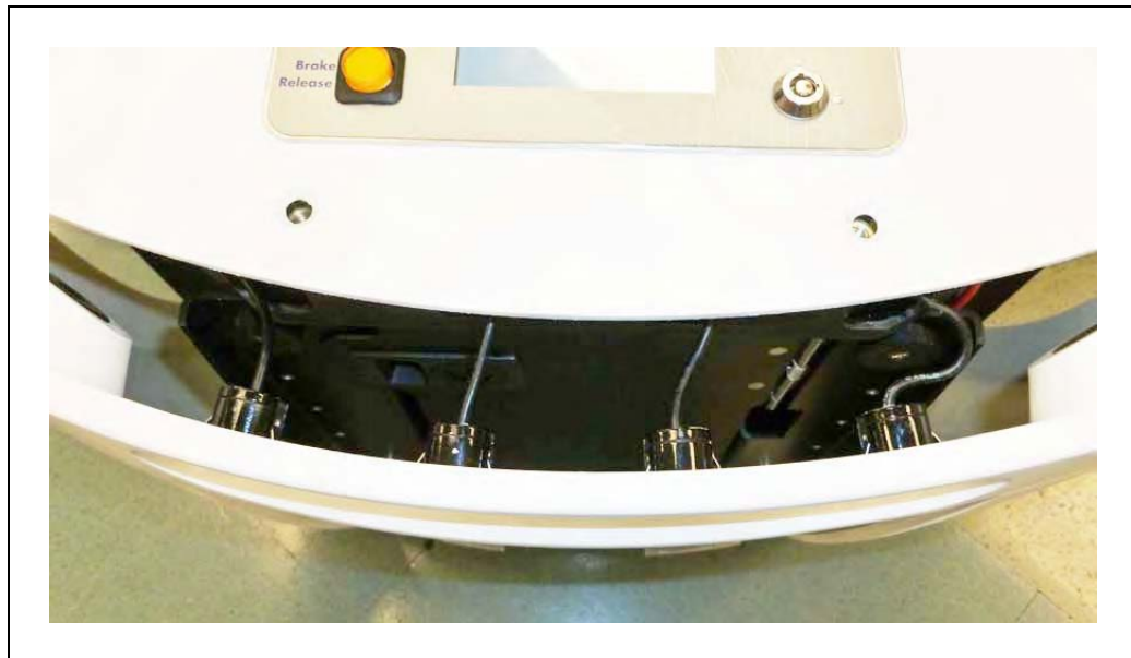
Figure 8-20. Sonar Leads, with Connectors Still in Chassis
