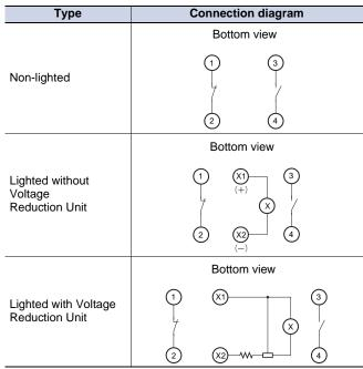
Note: The above terminal connection diagrams are examples for SPST-NO + SPST-NC.
