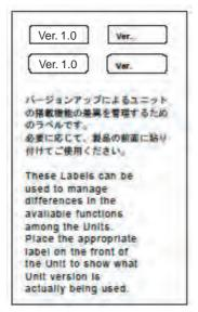
These labels can be attached to the front of previous CPU Units to differentiate between CPU Units of different unit versions.
