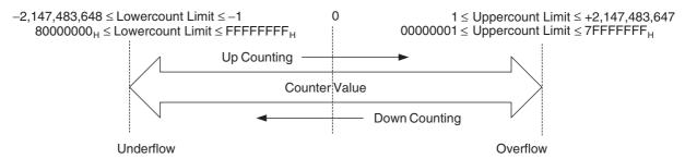
If the Counter Value goes above the Upper Count Limit or below the Lower Count Limit an Overflow- and Underflow flag will be set respectively. These are reported in CIO for the corresponding Counter.
