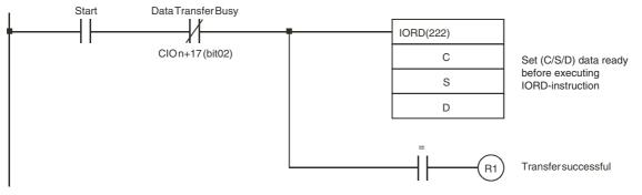
The Data Transfer Busy bit (CIO n+17, bit 02) is ON when the Unit is busy completing an IOWR/IORD-instruction or being initialised. When this bit is OFF the Unit is ready to execute the IORD-instruction. If an error occurs during the execution of the IORD-instruction the ER-flag turns ON.
