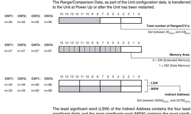
The least significant word (LSW) of the Indirect Address contains the four least significant digits and the most significant word (MSW) contains the most significant digit of the Indirect Address (refer to section the examples on the following pages).
