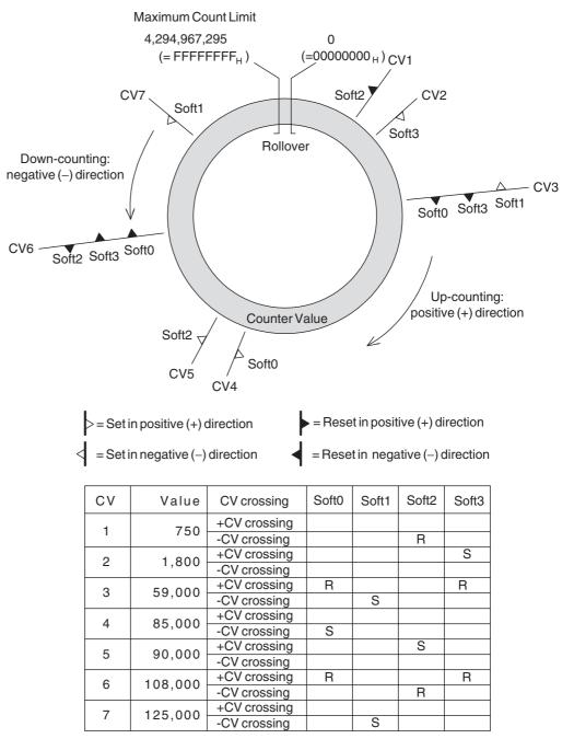
This example shows the Comparison Mode applied to a Circular Counter.
