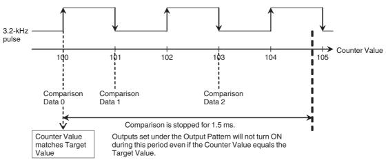
Comparison Stoppage for IOWR- and IORD-instruction Execution Comparison is stopped during the execution of IOWR/IORD-instructions and remains stopped until the processing of the instruction has been completed. The Data Transfer Busy bit is ON during this time.
