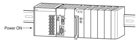
4. Create the I/O table. The I/O table can be created by using CX-Programmer Support Software or a Programming Console.
