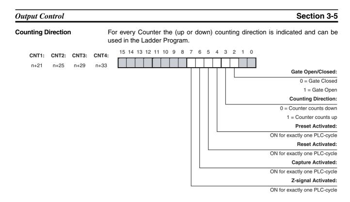
The Reset, Preset, Capture and Z-signal Activated Bits are ON for exactly one PLC-cycle after the occurrence of a (short) pulse which was detected since the previous I/O Refresh.
