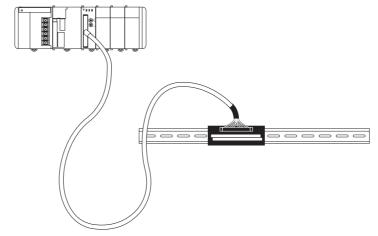
Refer to section Appendix A *Using Input Terminal Block Units* for information on the numbering of the screw-terminals. You need this information in case you want to connect the external signals via Terminal Block Units to the Counter Unit.
