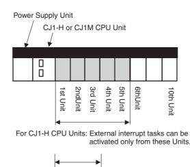
For CJ1M CPU Units: External interrupt tasks can be activated only from these Units.
