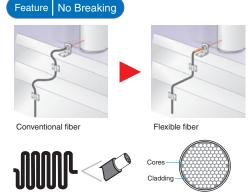
A large number of ultrafine cores are all surrounded by cladding. As a result, the fiber is flexible and can be bent without significantly reducing the light intensity. This helps solve problems, such as fiber being broken by getting caught on other objects.
