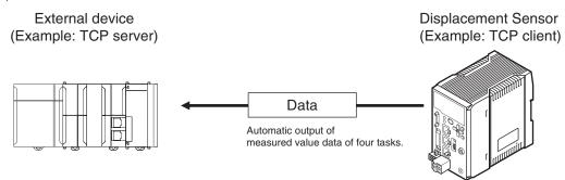
Data can be output with Ethernet or with RS-232C. Measured value data can be sent to an external device (e.g. PLC) serially (continuously) in ASCII format or binary format. External device There is no handshaking for whether or not an external device (e.g. PLC) can receive data.
