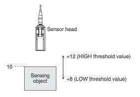
Example 3: Measure the level difference of the sensing object (execute zero reset at every measurement)
