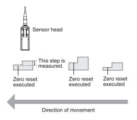
The zero reset function also allows setting the reference value to the hold value for a hold measurement or any value other than zero.
