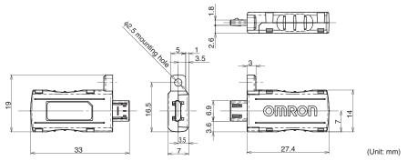
\* This comes with the Sensor Head (ZW-S07/S20/S30/S40/SR07/SR20/SR40). Be sure to use a Calibration ROM together with the Sensor Head with the same serial number.
