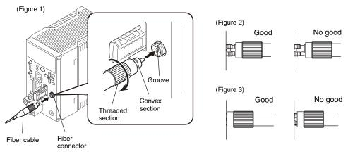
In the "No good" status in figure 2 and figure 3, optic signals cannot be transmitted and correct measurement is not possible. Always check that the system is in the "Good" status.
