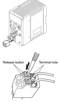
**2** Push in and hold the release button next to the terminal hole using a screwdriver while pushing the wire fully into the terminal hole and remove the screwdriver.
