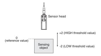
Example 2: Use the measured value according to the height of the sensing object (set 10 as an offset value)
