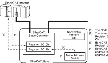
The Node Address Switch is set at power OFF. The value of Node Address Switch is applied to Register: 0012 hex, when the slave power is ON.
