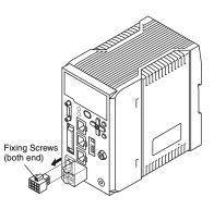
**2** Push in and hold the release button next to the terminal hole using a screwdriver while pushing the wire fully into the terminal hole and remove the screwdriver.
