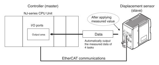
With EtherCAT communications, communications is performed via the I/O ports of the following four area on the Controller. Sysmac error status area I/O ports are used only when an NJ series CPU unit is connected as the master.
