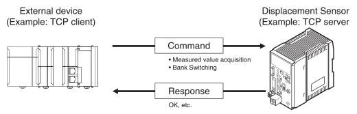
In actual terms, an ASCII character command (e.g. "MS" for acquiring the measured value) is issued from the external device (e.g. PLC). The displacement sensor returns responses such as "OK", "NG" or a value.
