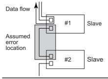
\*2. If a slave AL status error occurred together, a problem may have occurred in the wiring between the node where the slave AL status error occurred and the slave with out data connected to the upstream, making communication unstable. If there is no problem in the wiring, one of the slaves may have failed.
