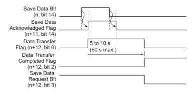
When saving data is completed, Data Transfer Completed Bit (word n+12, bit 2) turns ON.
