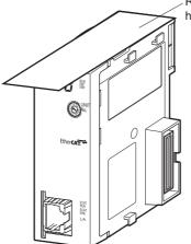
Remove the label after wiring has been completed.
