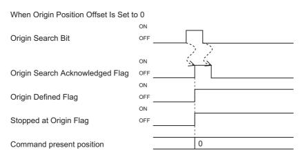
If you set the Origin Position Offset parameter to 0, the Stopped at Origin Flag also turns ON when the Origin Defined Flag turns ON.
