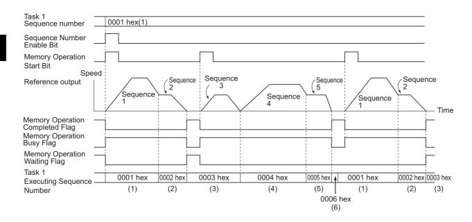
If you execute memory operation again while Sequence Number Enable Bit is OFF, the sequence number that is executed is the same as for a Memory Operation Individual Start Bit.
