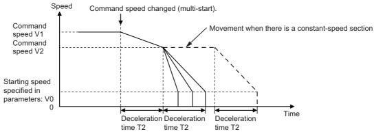
First, the axis decelerates to command speed V2 over deceleration time T2. When the movement distance is short and it would exceed the specified distance if the axis decelerates over deceleration time T2, the deceleration time changes according to the movement distance. In other words, the axis decelerates over a time that is shorter than the specified deceleration time.
