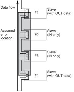
If only Process Data Reception Timeout is registered in the error log, an error location cannot be identified. Check the behavior of the network while changing the configuration to identify an error location.
