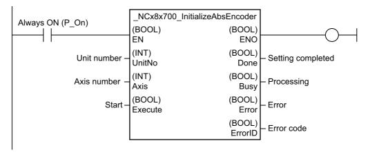
The absolute encoder can be set up by specifying the unit number and axis number in the function block and then turning ON the Start Bit.
