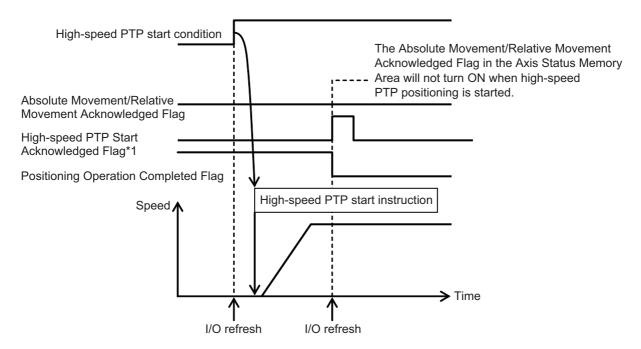
\*1 The High-speed PTP Start Acknowledged Flag will turn ON for at least one cycle from the I/O refresh period immediately after the PCU acknowledges the High-speed PTP Start Bit. This flag also shows the response status for a high-speed PTP start command. It can therefore turn ON more than one cycle after the flags that indicate axis operating status, such as the Axis Busy Flag.
