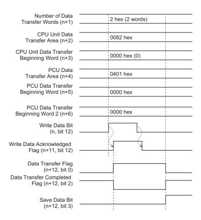
When data writing is completed, the Data Transfer Completed Flag (word n+12, bit 2) will turn ON. If an error occurs when data is written, the Data Transfer Invalid Flag (word n+12, bit 1) will turn ON and the error code will be output to word n+14.
