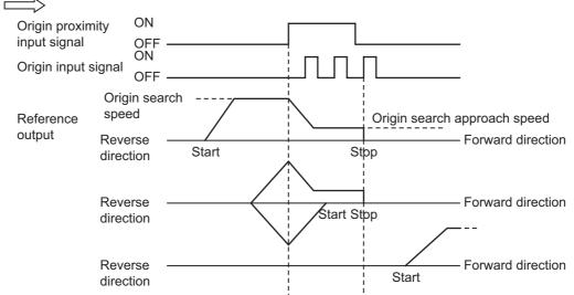
Origin Search Start Direction Different from Origin Input Detection Direction
