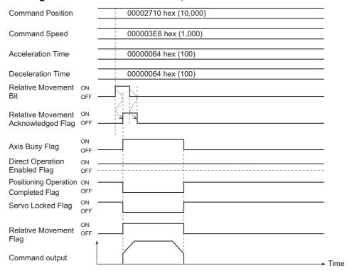
Example 2: Changing the Command Position to an Absolute Position of 10,000 Pulses during an Absolute Movement to 10,000 Pulses
