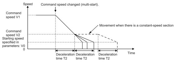
First, the axis decelerates to command speed V2 over deceleration time T2. When the movement distance is short and it would exceed the specified distance if the axis decelerates over deceleration time T2, the deceleration time changes according to the movement distance. In other words, the axis decelerates over a time that is shorter than the specified deceleration time.
