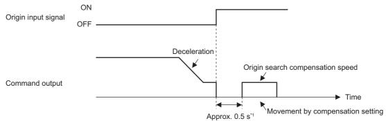
\*1. If you use the Deviation Counter Reset Bit, origin compensation operation starts approx. 0.5 seconds after the Deviation Counter Reset Bit turns OFF.
