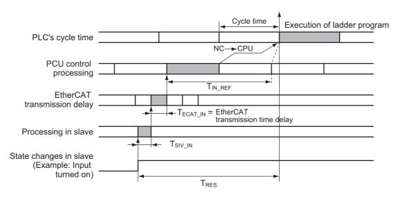
Processing time taken until the state change acquired from the slave is sent over EtherCAT communications link:
