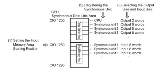
Next, set the I/O data type of the Synchronous Data Link from the synchronous unit using the PCU's parameters.
