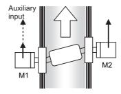
You can compensate the axis position temporarily by providing the auxiliary position input value if the position deviation occurs.
