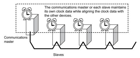
All devices perform control operations based on the distributed clocks to synchronize all devices. When the PCU is used with OMRON G5-series Servo Drives, distributed clocks are used for synchronization.
