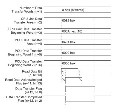
When data reading is completed, the Data Transfer Completed Bit (word n+12, bit 2), which is the same as for writing data, turns ON.
