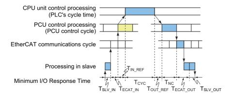
T<sub>SLV\_IN</sub> + T<sub>ECAT\_CYC</sub> + T<sub>CYC</sub> + T<sub>NC</sub> + T<sub>ECAT\_CYC</sub> + T<sub>SLV\_OUT</sub>
