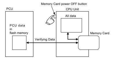
When this procedure is performed, the data on the Memory Card and the data in the internal flash memory of the PCU are compared.
