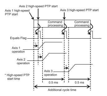
Although the high-Speed PTP positioning for axis 2 is executed immediately after the start of the high-Speed PTP positioning for axis 1, the time for executing the instruction increases by 0.5 ms. The high-Speed PTP positioning for axis 3 is executed after the completion of the high-Speed PTP positioning for axis 3 (that is, after a lapse of the time for executing the instruction).
