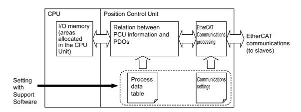
The process data table is provided to devices that are supported by the PCU as unique PCU setting information. The information settings in both the process data table and communications setting information are made in the PCU from the Support Software.
