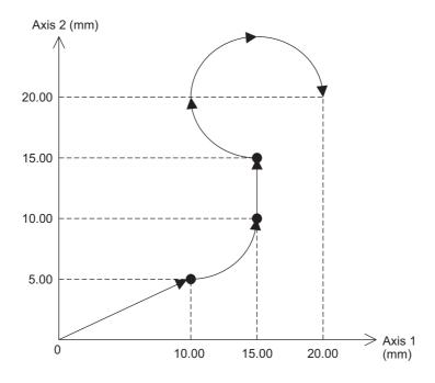
1) When you turn ON the operation start switch at the origin, the axes move to the point (10.00 mm, 5.00 mm10.00mm) via linear interpolation.
