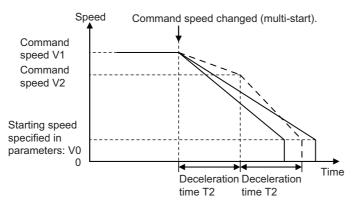
The axis starts decelerating to a stop based on the movement distance specified when multistarting is implemented.
