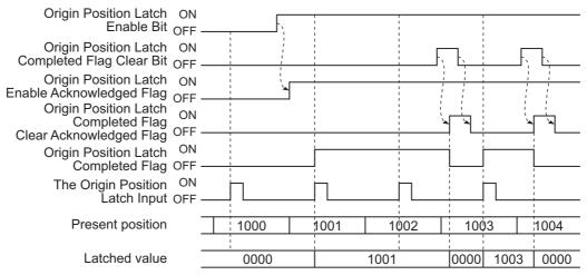
When the Interrupt Input Mask/ Origin Position Latch Enable Bit is OFF, the present position is not latched even if there is a latch input.
