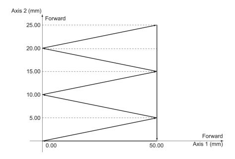
1) When you turn ON the operation start switch at the origin, the axes automatically perform positioning with linear interpolation in the following sequence and then stop:
