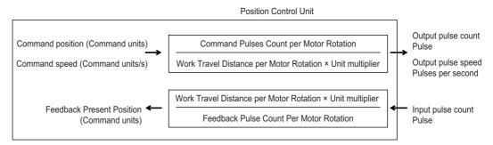
The command position after converted into pulses is a signed 32-bit value between - 2,147,483,648 and - 2,147,483,647. Similarly, the command speed is up to 1,048,576 pps after converted into pulses per second.
