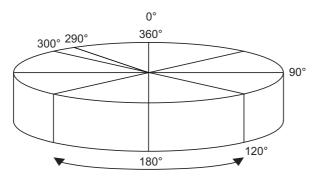
The shorter rotation direction is used for positioning.
