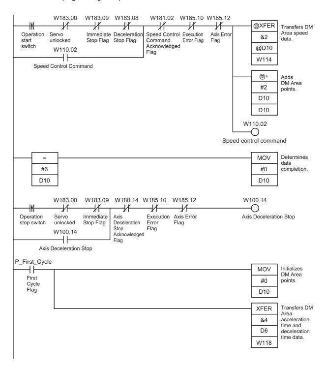
This programming example uses the Deceleration Stop Bit in the Manual Operation Command Memory Area to execute a deceleration stop on the Servo Drive which is registered for axis 1.
