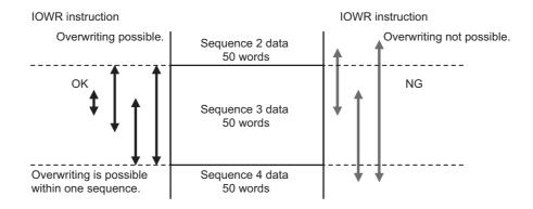
When you transfer cam table data with the IOWR(223) instruction, you cannot transfer data that contains data for more than one cam data. A warning will occur if data for more than one cam data is transferred.
