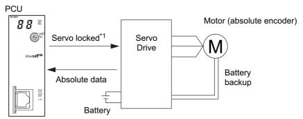
\*1 With unit version 1.4 or later, you can select the origin establishment timing with a common parameter For details, refer to the following function description.
