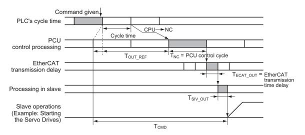
Maximum time between when an end refresh occurs on the cycle in which a command is executed from the user program and when the PCU actually acknowledges the command:
