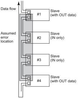
If only Process Data Reception Timeout is registered in the error log, an error location cannot be identified. Check the behavior of the network while changing the configuration to identify an error location.
