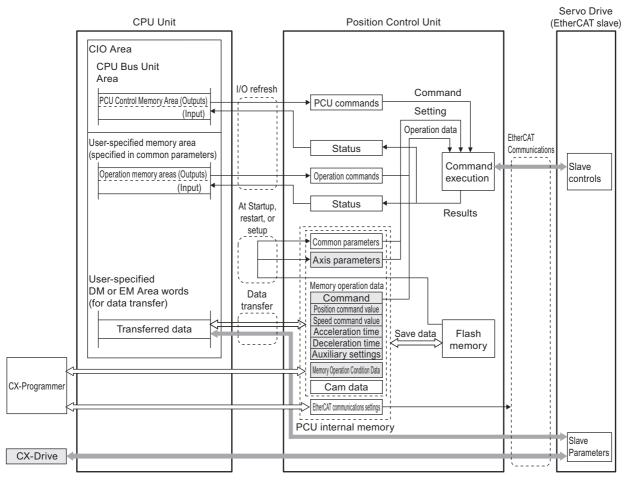
■: The shaded areas are used when a G5-series Servo Drive is connected.
