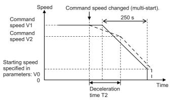
With a fixed deceleration time of 250 seconds, the axis does not decelerate immediately when you implement multi-starting and the movement distance is adjusted by using the constant-speed section.
