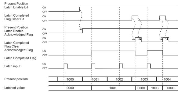
When the Interrupt Input Mask/ Present Position Latch Enable Bit is OFF, the present position is not latched even if there is a latch input.
