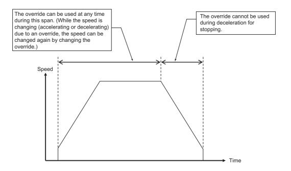
If you change the override value during operation, the axis accelerates/decelerates to the target speed that reflects the override value. If a constant acceleration/deceleration rate is specified for the Acceleration/Deceleration Time Selection, the axis will start to accelerate/decelerate toward the changed speed as soon as the override is changed.
