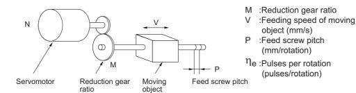
The following formula gives the travel distance per pulse relative to the motor driver. This is called the pulse rate.
