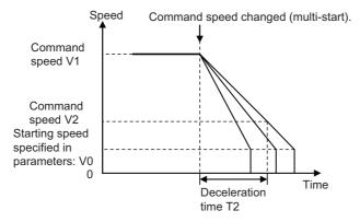
The axis starts decelerating to a stop based on the movement distance specified when multistarting is implemented.
