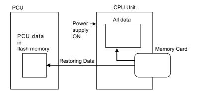
When this procedure is performed, the PCU data file on the Memory Card is read and the data is restored to the PCU.
