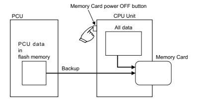
When this procedure is performed, a PCU data file is created and written to the Memory Card along with other backup files.
