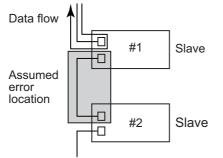
\*2. If a slave AL status error occurred together, a problem may have occurred in the wiring between the node where the slave AL status error occurred and the slave with out data connected to the upstream, making communication unstable. If there is no problem in the wiring, one of the slaves may have failed.
