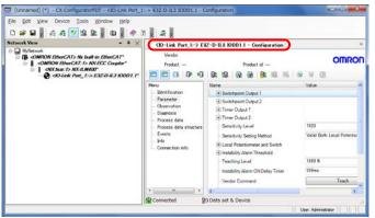
15 Select Observation listed under Menu on the <IO-Link Port\_1:-> E3Z-D-IL3 IODD1.1 - Configuration Tab Page.
