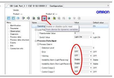
Oheck that Operation mode switch on Photoelectric Sensor is set to Light ON (factory setting).
