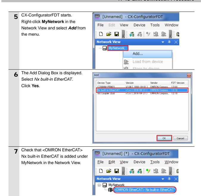
Right-click **<OMRON EtherCAT>**Nx built-in EtherCAT and select
