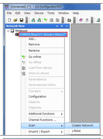
The Lifelist Dialog Box is displayed after completing the network scan. Check that <OMRON EtherCAT:1> NX-ECC Coupler is added under Nx built-in EtherCAT.
