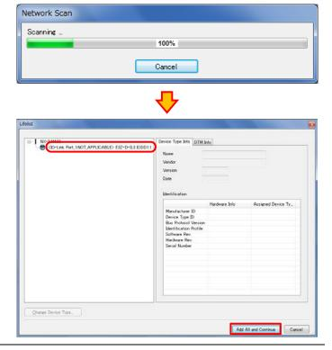
11 Check that the network configuration is created in the Network View as shown on the right.
