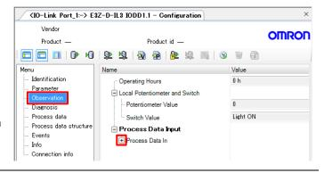
Click the <sup>™</sup> icon (Enable or disable cyclic read from device for dynamic variables) on the <IO-Link Port\_1:-> E3Z-D-IL3 IODD1.1 - Configuration Tab Page.
