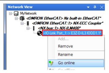
13 Check that Photoelectric Sensor is connected online.
