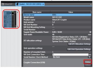
(4) Right-click **Unit 0** (EtherCAT Coupler Unit) after checking the online connection. Select *Clear All Memory* from the menu.
