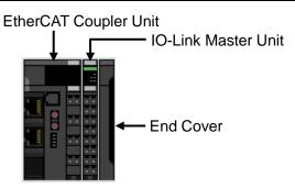
Check the position of the hardware switches on EtherCAT Coupler Unit by referring to the figure on the right.
