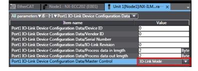
\*If IO-Link Mode is not displayed in the *Value* Column, select the mode from the pull-down list.
