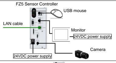
3 Connect FZ5 Sensor Controller to Switching hub with LAN cable.
