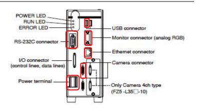
As shown in *5.2. Device*Configuration, connect Camera,
