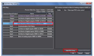
Register the output points of the connected SmartSlice Analog Output Unit.
