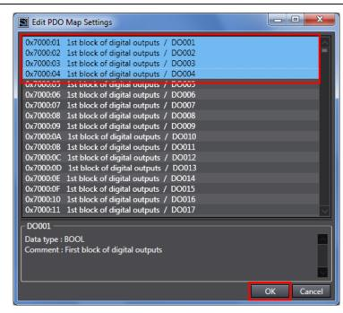
5 Confirm that D0001 to D0004 are registered in the PDO entries included in 1st block of digital outputs D0001 to D0240.
