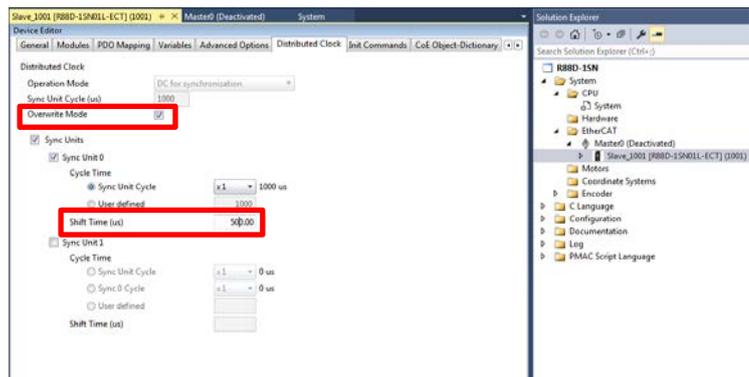
Correspondence between the servo frequencies of the Controller and the Shift Time values is as follows:
