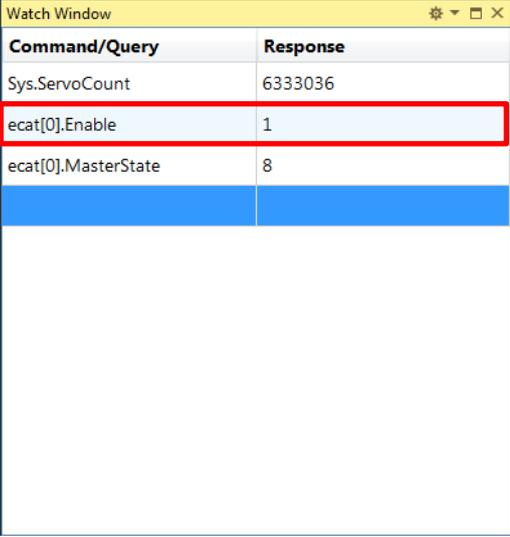
A "Watch Window" table with two columns: "Command/Query" and "Response". The rows are: "Sys.ServoCount" with response "6333036", "ecat[0].Enable" with response "1" (highlighted with a red box), and "ecat[0].MasterState" with response "8".                                                                                                                                                                          |
