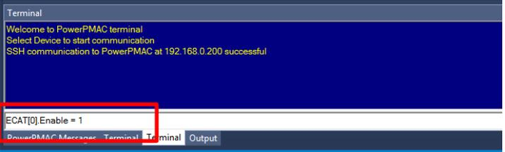
A terminal window with a dark blue background. The text reads: "Welcome to PowerPMAC terminal", "Select Device to start communication", "SSH communication to PowerPMAC at 192.168.0.200 successful". Below this, the command "ECAT[0].Enable = 1" is entered and highlighted with a red box. The terminal tabs at the bottom are labeled "PowerPMAC Messages", "Terminal", "Terminal", and "Output".                    |
