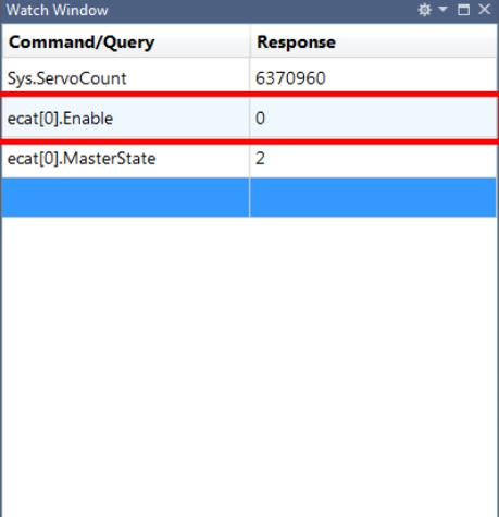
A "Watch Window" table with two columns: "Command/Query" and "Response". The rows are: "Sys.ServoCount" with response "6370960", "ecat[0].Enable" with response "0" (highlighted with a red box), and "ecat[0].MasterState" with response "2".                                                                                                                                                                         |
