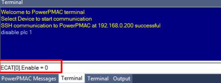
A terminal window with a dark blue background. The text reads: "Welcome to PowerPMAC terminal", "Select Device to start communication", "SSH communication to PowerPMAC at 192.168.0.200 successful", "disable plc 1". Below this, the command "ECAT[0].Enable = 0" is entered and highlighted with a red box. The terminal tabs at the bottom are labeled "PowerPMAC Messages", "Terminal", "Terminal", and "Output". |
