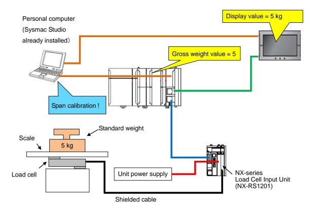
The steps to perform span calibration with the Sysmac Studio are as follows. Note that you can skip steps 1 and 2 when performing span calibration following zero calibration.
