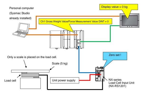
Following the above condition where zero set is performed, placing a measured material on the scale allows the weight value of the measured material to be checked from the I/O data, Ch1 Gross Weight Value/Force Measurement Value DINT and Ch1 Gross Weight Value/Force Measurement Value REAL.
