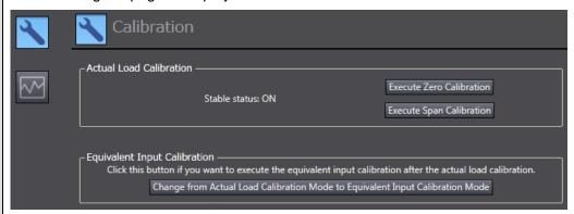
Click the Change from Actual Load Calibration Mode to Equivalent Input Calibration Mode Button in Equivalent Input Calibration.
