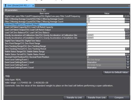
2 Since a 5 kg standard weight is used for calibration in this example, set the Ch1 Standard Weight to 5. Leave the other setting values of the Unit operation settings at their defaults.
