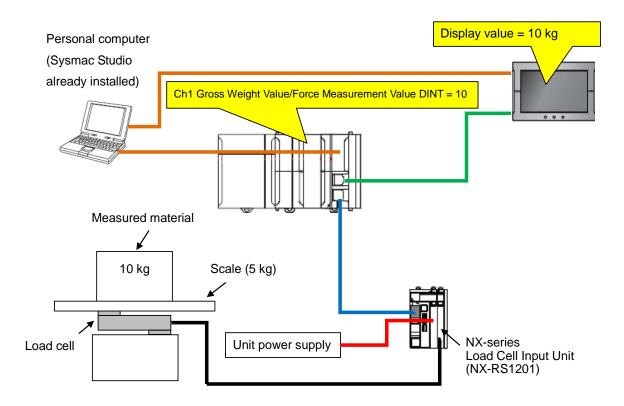
From the Sysmac Studio's I/O map, you can check the values of Ch1 Gross Weight Value/Force Measurement Value DINT and Ch1 Gross Weight Value/Force Measurement Value REAL. The following is how to check measurement values from the Sysmac Studio's I/O map.
