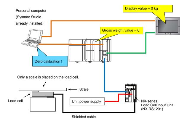
The steps to perform zero calibration with the Sysmac Studio are as follows.
