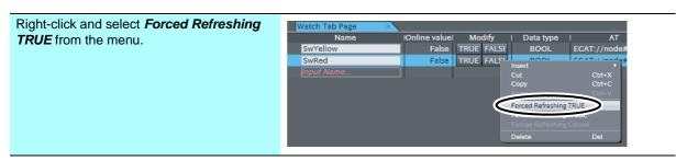
When the input value from the red pushbutton switch is forced to TRUE, the self-holding rung is reset and the yellow indicator goes out.
