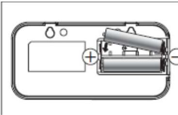
(2) Insert two batteries with careful attention to proper polarity.
