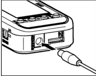
(1) Insert the plug of the AC adapter or DC power supply cable into the power supply input terminal.
