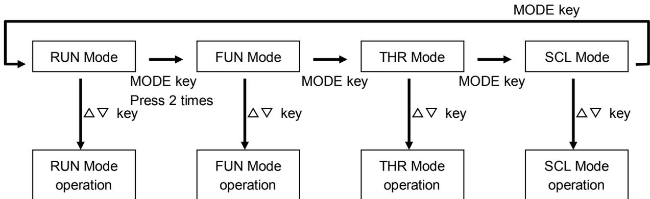
The Differential Pressure Station has four operation modes. These modes can be switched with the MODE key.
