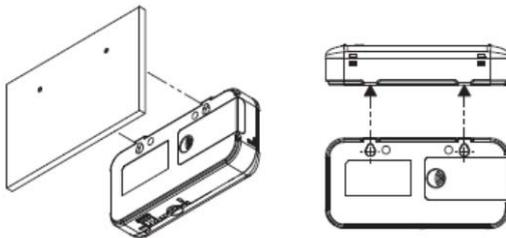
Use M3 screws to hook the screw head on the screw hook holes. Attach the device with an interval of 2.5 mm or more between the bottom of the screw head and the wall surface.
