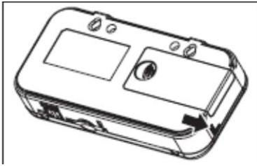
(1) Slide to open the battery cover on back of the main unit.
