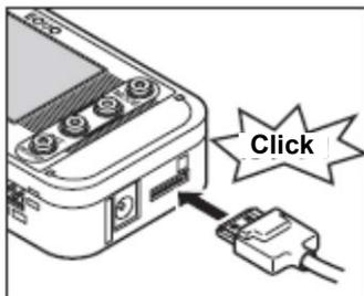
Insert the Sensor Head into the Sensor Head connector until it clicks.
