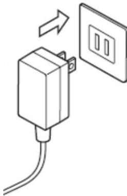
(2) When using an AC adapter, insert the plug of the AC adapter into an outlet. (100 VAC to 240 VAC).
