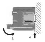
• Secure each DIN Track with at least three screws. DIN Track: PFP-50N (500 mm), PFP-100N (1,000 mm)
