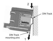
Push the Controller until it is mounted to the DIN Track.
