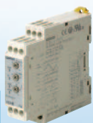
● Over and under voltage ● All-in-one configuration ● 3-/4-wire selection for 3-phase power supply ● Input range selection 3-Phase Voltage, Sequence, Loss Relay K8AB-PM
