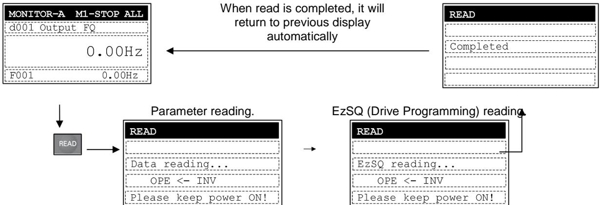
**NOTE:** All inverter parameters saved in LCD digital operator are overwritten after the **READ** key is pressed.
