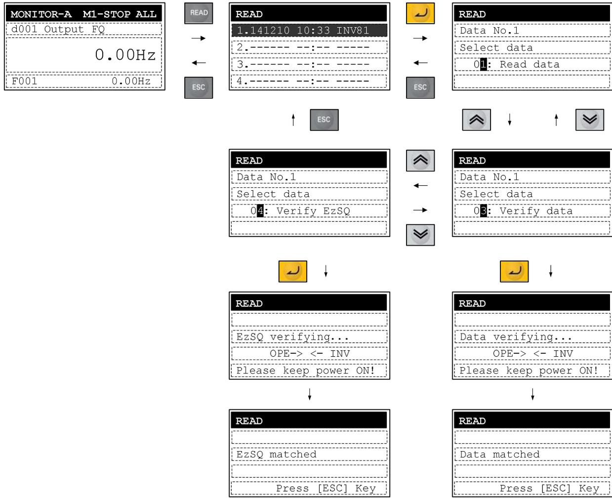
The result is shown automatically after the parameter or EzSQ (Drive Programming) verification is completed.
