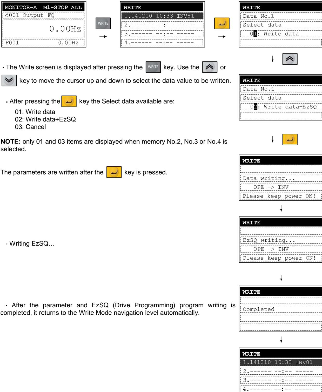
• The Write screen is displayed after pressing the **WRITE** key. Use the **↑** or **↓** key to move the cursor up and down to select the data value to be written.
