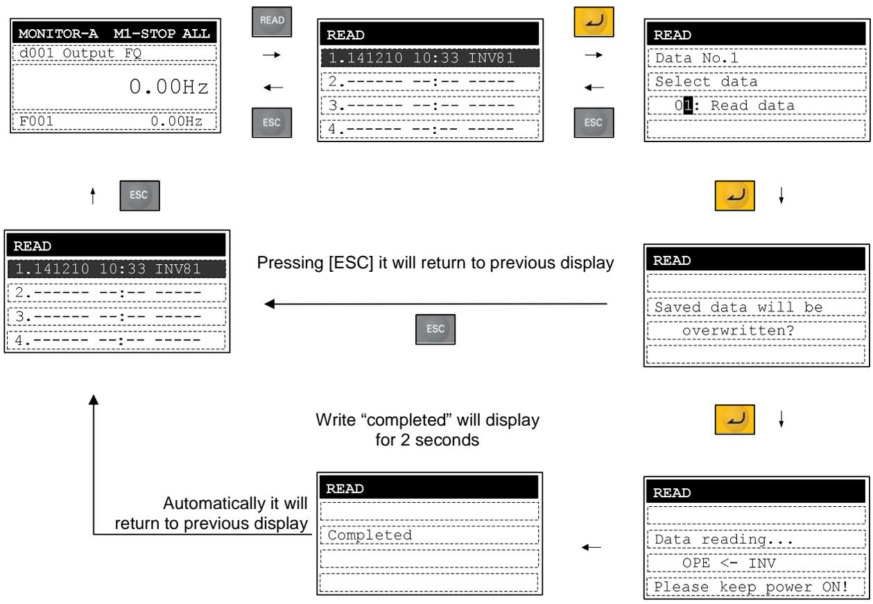
**When the inverter supports EzSQ (Drive Programming) function**
