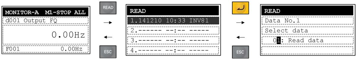
• In any display mode except Write Mode and Option Mode, the read screen is displayed after pressing the **READ** Key. If there aren't parameters stored in LCD digital operator, it will show "—".
