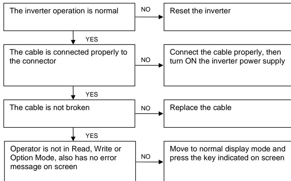
(3) If the operator screen becomes dark or characters cannot be identified, inductive noise may be entered from the cable. Separate LCD digital Operator cable more than 15cm from other cables. To reset the disturbed screen, turn ON any keys of LCD digital operator. If the same symptom appears again, turn OFF the inverter power supply or reset the terminal reset signal.
