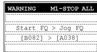
**NOTE:** When a trip happens, ALARM LED will be light on. Press the
