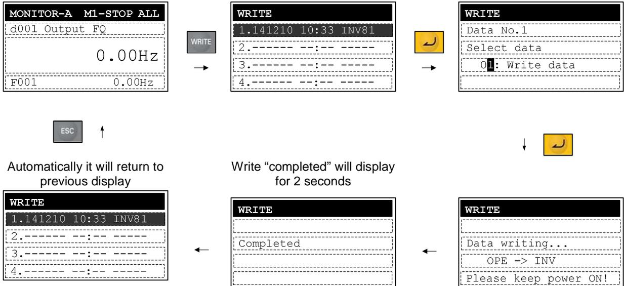
**When the inverter supports EzSQ (Drive Programming) function**
