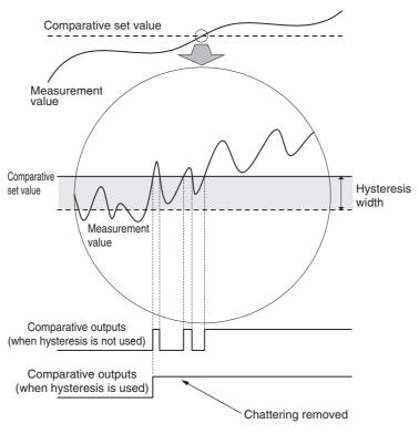
Hysteresis works in the direction of decreasing measurement values for comparative set values HH and H and works in the direction of increasing measurement values for comparative set values LL and L. However, hysteresis works in the direction of decreasing measurement values for all set values if the output pattern is set to a level output.
