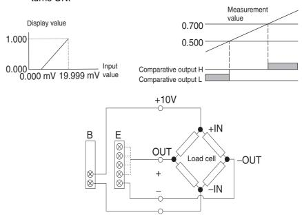
\* 2 mV/V indicates a load cell output of 2 mV for 1 V applied voltage for the rated load (when using a load of 1 N). When the applied voltage is 10 V, the load cell output is 20 mV (2 mV×10)
