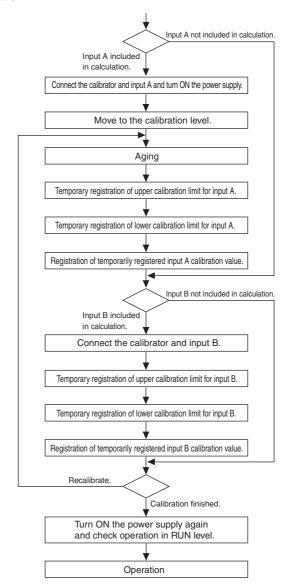
The input type that can be calibrated according to this flowchart is the type selected under "input type A" or "input type B." To calibrate other input types, switch the setting for "input type A" or "input type B" in the initial setting level to the desired input type and then perform calibration according to the flowchart outlined above.
