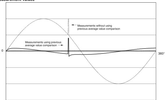
Previous average value comparison makes the measurement value the difference between the present input value and the average of all previous input values.
