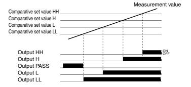
\* The PASS output turns ON when any of the HH, H, L, or LL output turns OFF.
