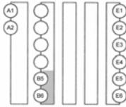
The following sensor power supply can be supplied from terminals B5 and B6.
