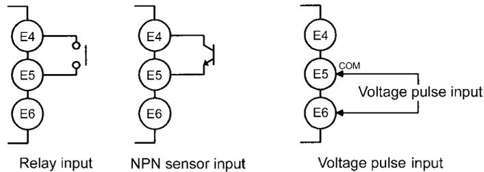
For the PNP sensor input connection, refer to "1-3 I/O Circuit".
