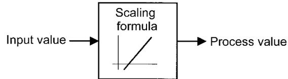
Scaling allows conversion of input values to process values in easy-to-understand notation.
