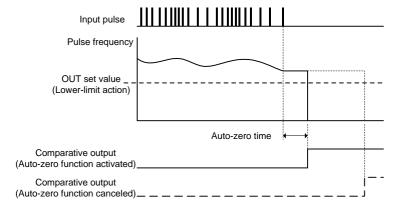
To eliminate such a situation, the product has an **auto-zero** function that shifts the input pulse frequency to zero forcedly when no pulse is received for a predetermined time.
