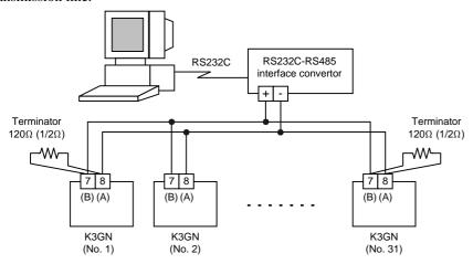
Match the communications format of the K3GN and the host computer. If a one-to-N system is being used, be sure that the communications formats of all devices in the system (except individual unit numbers) are the same.
