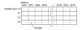
Append to each variable type an access-size-based address that is expressed in 2-byte hexadecimal code
