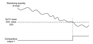
• Comparative output 1 turns on when the remaining quantity of soup decreases to 20%.
