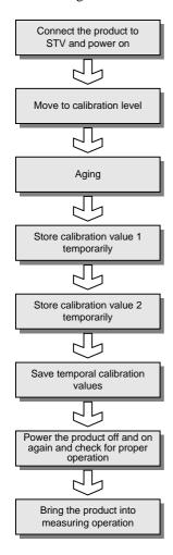
In the above flow, a range specified by the "analog range" parameter undergoes calibration.
