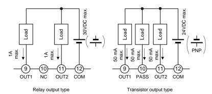
The  $\left(\begin{array}{c} \bot \\ \hline \end{array}\right)$  connection causes the current to flow in the direction opposite to indicated by the arrows.
