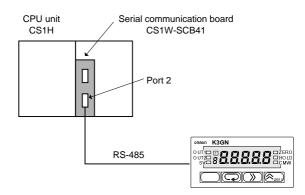
Set the TERM switch to "ON" and the WIRE switch to "2" and connect a terminator to the K3GN.
