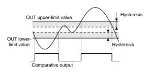
Combinations of comparative outputs 1 and 2 offer the possibility of producing a wide variety of actions including upper-limit + another upper-limit actions, lower-limit + another lower-limit actions, and two-level outside-the-range actions.
