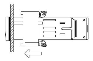
(4) Tighten the two screws of the adapter in alternate order to a tightening torque of 0.29 to 0.39 N·m.
