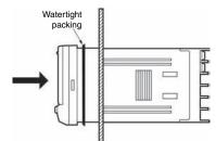
3. Insert the adapter into the grooves on the left and right sides of the rear case and push until it reaches the panel and is fixed in place.
