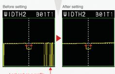
Lost part on a profile due to insufficient amount of light received
