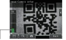
Adjust the brightness with the slider at the bottom of the display. You can also press [AUTO] to automatically set the brightness according to the image.
