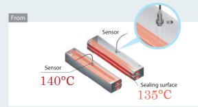
On a conventional sealing machine, temperature sensors can often be located too far away from the sealing surface, so a difference occurred between the temperature of the sealing surface and the temperature that was actually being controlled.
