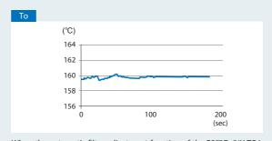
When the automatic filter adjustment function of the E5 $\square$ D /NX-TC is used, this periodic temperature variation is suppressed automatically. It becomes possible to perform stable temperature control.
