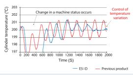
\* Data measured by OMRON on a water-cooled twin screw extrusion molding machine.
