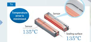
The installation position of the temperature sensor for packaging machines has been brought closer to the sealing surface to bring the temperature of the sensor closer to the temperature of the sealing surface. This minimizes the effects from variation in the surface temperature of the packaging materials.
