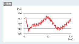
When a temperature sensor for a packaging machines is used, there is sometimes periodic temperature variation generated when there is a marked effect from the heat on the packaging materials side.
