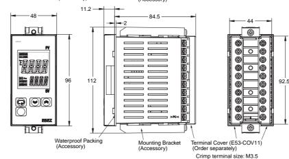
Note: To remove the Controller from the case, loosen the screw at the bottom of the front panel with a screwdriver while pressing down on the hook at the top of the front panel.
