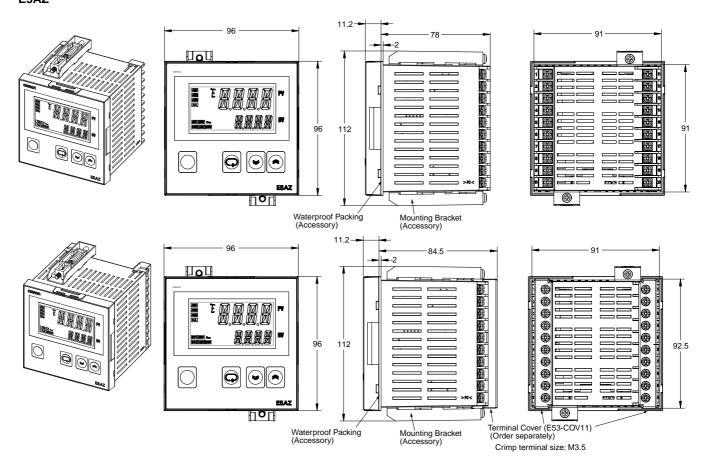
Note: To remove the Controller from the case, loosen the screw at the bottom of the front panel with a screwdriver while pressing down on the hook at the top of the front panel.
