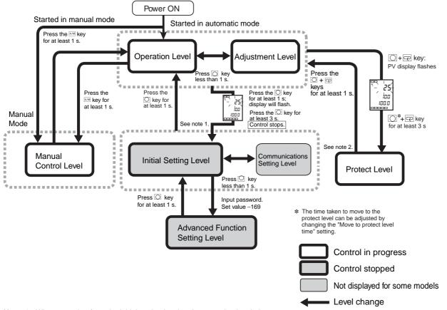
**Note: 1.** When returning from the initial setting level to the operation level, the default in the operation level will be displayed.
