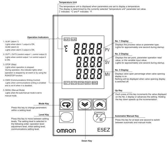
Each press of this key decrements values displayed on the No. 2 display or reverses the setting. Holding the key down speeds up the decrementation.
