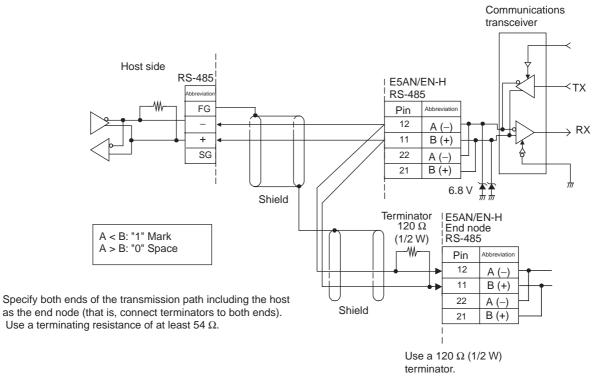
Match the communications specifications of the E5CN/AN/EN-H and the host. When using a 1: N connection, set the same communications specifications in all of the Units. (Of course, each Unit must have a unique unit number.) This section explains how to set the E5CN/AN/EN-H's communications specifications. For details on the host, refer to the User's Manual provided with the host.
