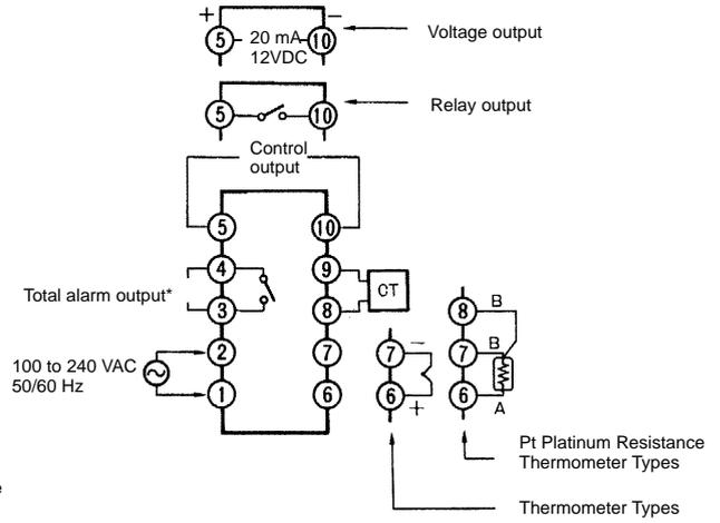
\*The total alarm output goes ON when either the alarm or the burnout alarm is activated.
