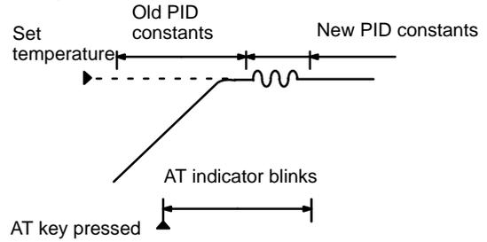
The optimum PID constants are calculated by this method by varying the control output variable and generating external oscillation.
