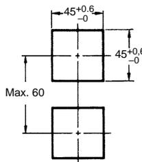
Side-by-side Mounting of N Temperature Controllers
