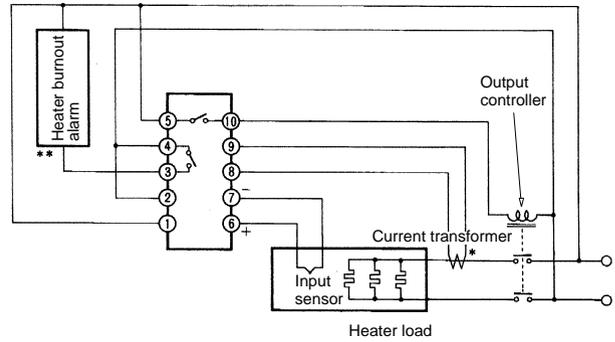
\*This wiring must be passed through the hole of the Current Transformer. The Current Transformer can be connected to the sensor in any polarity
