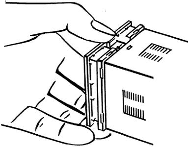
2. The following switches must be set: the temperature sensor selector, the operating mode selector, and the alarm mode selector. There is also a protection switch that can be set to protect settings. The following figure shows the locations of internal switches on the internal mechanism.
