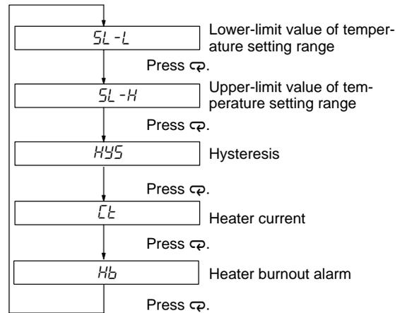
Of the above parameters, only the hysteresis, which is described below, differs from the parameters for PID control. Refer to 1. *PID Control* for details on other parameters.
