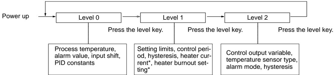
\*These are displayed only with Heater Burnout Alarm Types.
