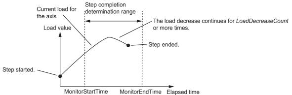
It is determined that the step is completed when *MonitorStartTime* = *MonitorEndTime*, regardless of the elapsed time from the start of the step.
