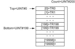
If there are already 20,000 trace records stored in *PrgOprTraceRecorder* and another trace record is added, the oldest trace record is overwritten. The values of the variables when the 20,001st trace record is added are as shown in the following figure.
