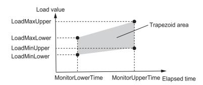
You can set the current position of the axis as the reference type to evaluate outside the time elapsed from the execution of this function block. To do so, read the above figure as if *MonitorUpperTime* were replaced with (*MonitorUpperPos* + *PrgLoadAlarm.InPosWidth*) and *MonitorLower-Time* as if it were replaced with (*MonitorLowerPos* – *PrgLoadAlarm.InPosWidth*).
