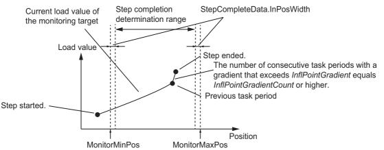
It is determined that the step is completed when *MonitorMinPos* = *MonitorMaxPos*, regardless of the current position of the monitoring target.
