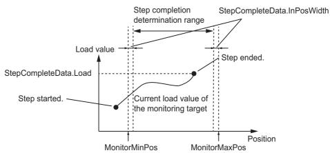
It is determined that the step is completed when *MonitorMinPos* = *MonitorMaxPos*, regardless of the current position of the monitoring target.
