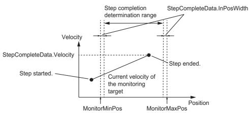
It is determined that the step is completed when *MonitorMinPos* = *MonitorMaxPos*, regardless of the current position of the monitoring target.
