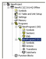
As shown below, SFC programs can be created in interrupt tasks and executed as extra tasks. Refer to the SYSMAC CS/CJ Series Programmable Controllers Programming Manual (Cat. No. W394) for information on extra tasks.
