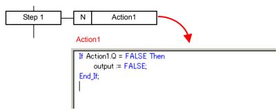
When step 1 has become inactive, action flag Action1.Q goes OFF, the action flag (Action1.Q) becomes FALSE, and the output goes OFF.
