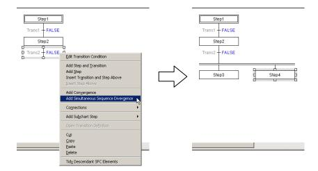
A simultaneous sequence divergence and 2 subsequent steps will be added.
