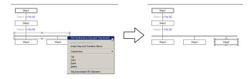
A step is added to the simultaneous sequence divergence.
