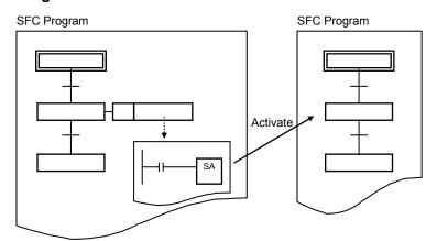
**Note:** If the SA step control instruction is used to activate another step in the same SFC program from an action ladder program in the SFC program, the activated step's action will be executed in the next cycle.
