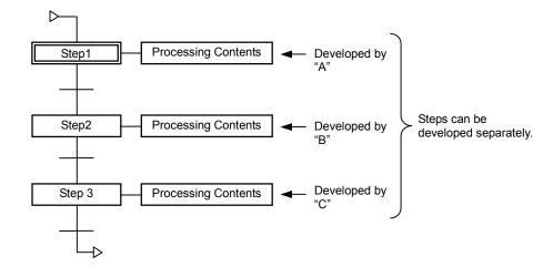
Programs are independently completed for each step, and are therefore simple to reuse
