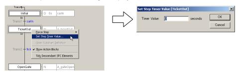
3 On the Set Step Timer Value dialog, input the desired timer value (0-65535 seconds or 0-6553.5 seconds) and click **OK**. The new value is reflected on the PLC.
