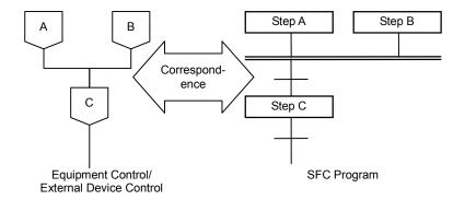
Programs can be created separately for each step, without the need to consider complicated requirement exchanges between steps. In other words, each step can be programmed separately, by a different developer, making program development simpler and more efficient.
