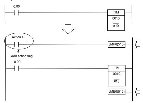
When you do not want a timer/counter PV refreshed after the step becomes inactive in timer/counter instruction processing like the processing in the chart shown above, add the action flag by ANDing the flag as a NO execution condition to a JUMP (JMP0) instruction, and enclose the timer/counter instruction between JMP0 and JME0. Even if the final scan is executed, the PV will not be refreshed additionally.
