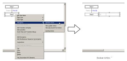
An action block is inserted to the right of the step.
