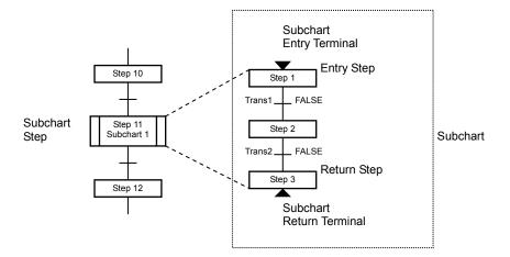
A subchart is called up by a subchart step. Its execution begins at the subchart entry terminal, and returns to the main process flow at the subchart return terminal.
