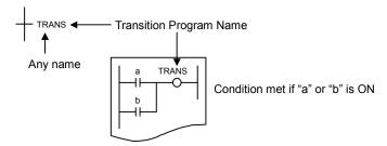
When a transition program is used as a transition condition, specify a transition program name for the transition condition. If a conditional equation is specified with a different Boolean variable name, than that of transition program name for the transition condition, the program will not run properly.
