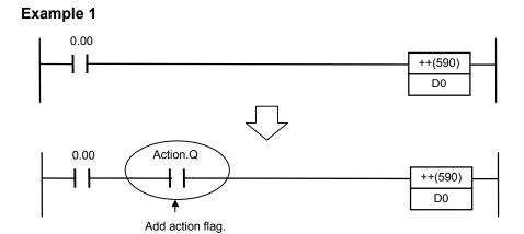
With processing such as the increment processing shown above, add the action flag by ANDing the flag as a NO execution condition. Even if the final scan is executed, the value of D0 will not be incremented in the final scan.
