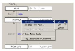
The step will be marked to indicate that it has been force-set/force-reset, as shown below.
