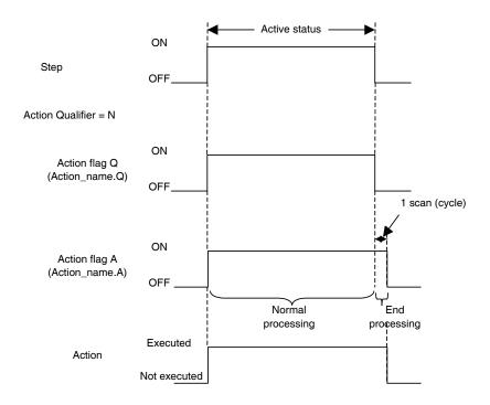
The following diagram shows the operation of the action flags when the final scan function was disabled by clearing the *Apply Final Scan Logic* Option on the General Tab Page of the SFC program's Property Dialog Box.
