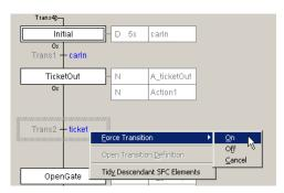
The transition will be marked to indicate that it has been force-set/force-reset, as shown below.
