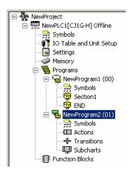
As shown below, SFC programs can be created in interrupt tasks and executed as extra tasks. Refer to the SYSMAC CJ Series CJ2 Unit Software User's Manual (Cat. No. W473) and the SYSMAC CS/CJ Series Programmable Controllers Programming Manual (Cat. No. W394) for information on extra tasks.
