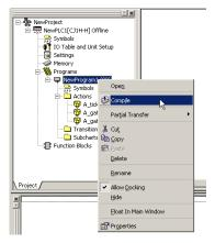
The check results for the program will be displayed on the **Compile** tab of the output window.
