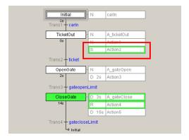
\*4: If an action has an S-series AQ (S, SL, SD), its activity status can be monitored, even while the action blocks are hidden.
