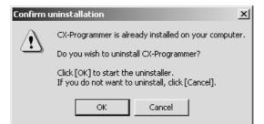
Click the **OK** Button and uninstall the earlier version of the CX-Programmer. If the <u>Cancel</u> Button is clicked, CX-One installation will continue without uninstalling the earlier version of the CX-Programmer. This would result in there being two versions of the CX-Programmer installed at the same time, so we recommend always clicking the **OK** Button.
