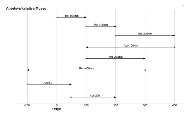
An absolute move, tells the SmartStep, where the move should end, in relation to a fixed origin position (Position 0)
