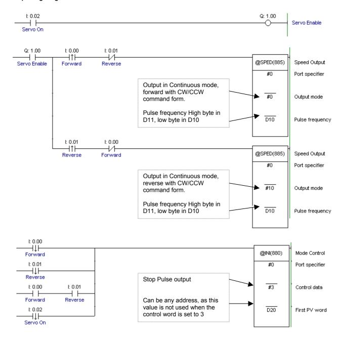
Ensure that the value in D10 and D11 is written prior to executing the above code by including a move value in for example a first scan contact
