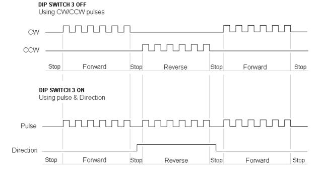
NOTE: When using the pre-assembled cables with the CJ1M PLC's, only CW/CCW command mode is available.
