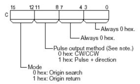
Note: Use the same pulse output method when using both pulse outputs 0 and 1.
