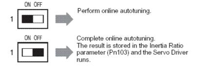
Online Auto tuning attempts to calculate the load inertia at the motor shaft. In order to do this, the motor speed must be above 500 rpm and the load torque must exceed 50%. Auto tuning is normally performed by repeatedly applying a high-speed step type movement in first one direction, then the other. The SmartStep can then dynamically calculate the load inertia.
