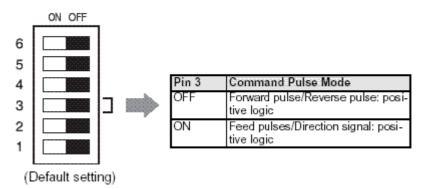
CC/CCW command form uses each channel of the pulse train input to determine the amount of movement (the number of pulses received) and the direction in which to move (the channel on which the pulses are received)
