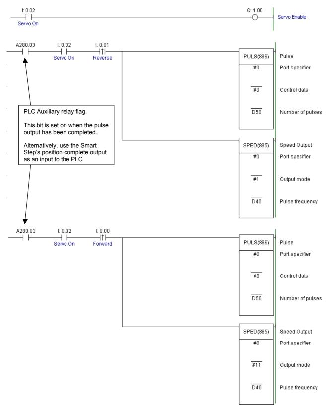
A280.03 is a PLC status bit, which is high when the PLC is not outputting pulses, i.e. a move is considered complete within the controller. If the SmartStep gain is low, then the motor may still be moving to its final position. Using the Position complete bit from the SmartStep is an indication that the SmartStep is within a 'window' of the final position. The width of this window is set by SmartStep parameter Pn500 and can't be changed by Dip Switch settings.
