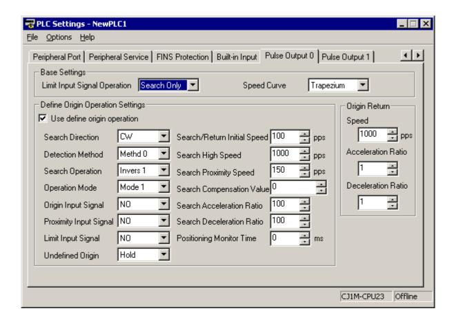
Unless the settings are made in the PLC, the ORG instruction cannot be used. The Use define origin operation checkbox is not made effective until the PLC is next powered up.
