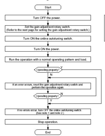
Do not perform extreme adjustment and setting changes as they may destablize the operation. Adjust the gain a little at a time while checking the Servomotor operation.
