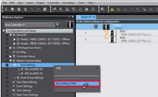
Edit axis settings according to the XY stage ball screw system
