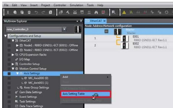
**Axis number** has been set to 0 and 1, **Axis type** to Servo axis and **Output device 1** to Node: 1 and Node: 2 on CH1 (Channel 1).
