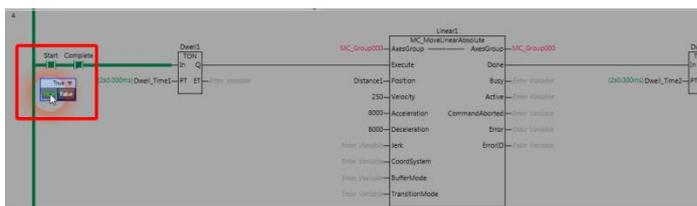
Linear1 is executed and positioning is started for both axes. When the positioning for Linear1 is completed, linear1 execution stops and Linear2 is executed. This operation is repeated with 2 seconds Dwell time between each movement.
