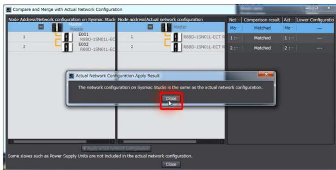
Confirm the detected configuration and close the window
