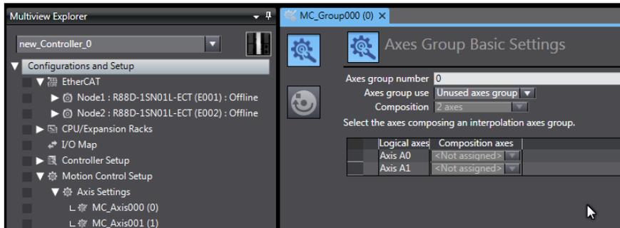
Set the Axes Group Basic Settings for axes group 0 as shown in the following figure.
