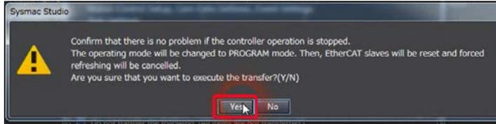
The operating mode changes to PROGRAM mode, and the Sysmac Studio starts transferring the project to the CPU Unit. During the transfer, a progress bar appears in the Synchronize Pane.
