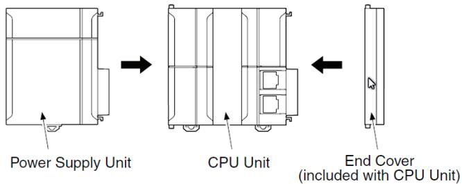
After joining the connectors between the Units, use the sliders at the top and bottom of each Unit to lock the Units together. Lock the sliders firmly into place.
