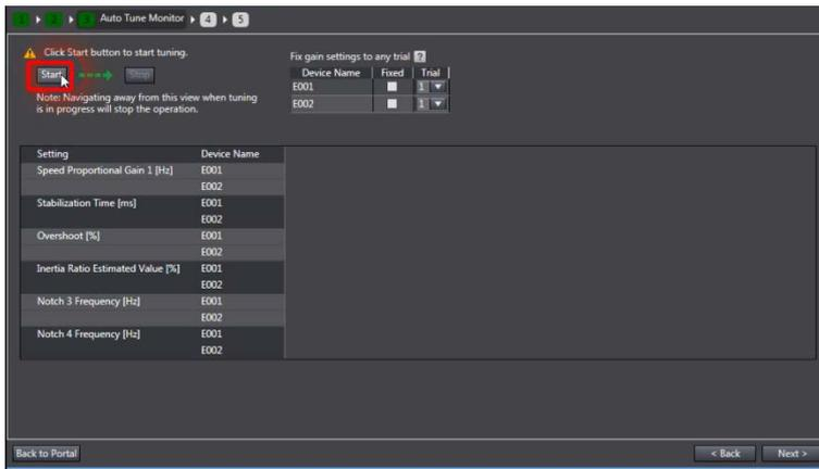
Gain will be increased gradually until achieving the specified settling time. The positioning window, specify the position deviation to determine that the positioning is completed. If it detects a vibration above the vibration detection level during tuning, an adjustment failure will occur.
