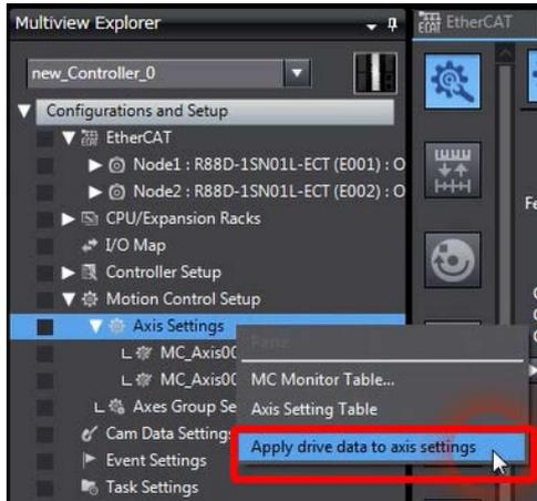
Click the **Yes** Button to acquire data from the servo drive via EtherCAT Network
