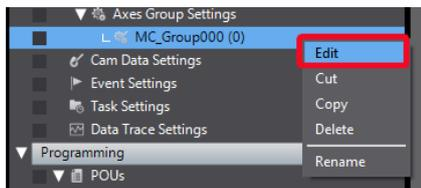
The axes group settings are displayed on the Axes Group Basic Settings Display in the Edit Pane.
