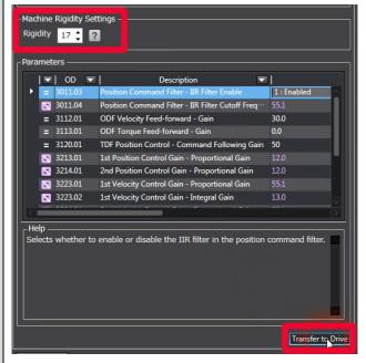
Push transfer to send the gain parameters to the drive.
