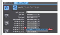
This will assign node 1 and the drive to the input device for axis 0.
