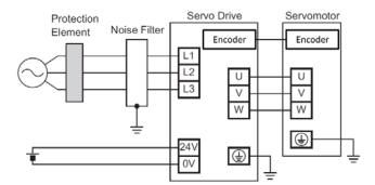
Here is an example servo drives with its capacity 3 kW or less.
