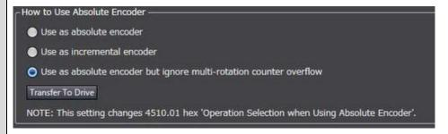
1S motor has an absolute encoder for all models. But it can be used as incremental if needed. When using Sysmac Controller, it is recommended to keep the default value. (as described in previous step 3)
