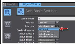
4. Select the Servo Drive to use in the Input device Box
