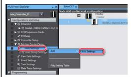
Axis 0 is added to the Multiview Explorer. The axis is added as MC\_Axis000.
