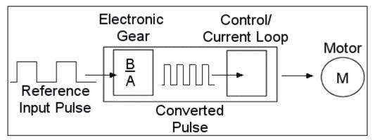
Figure 59: Illustration of Gear Function
