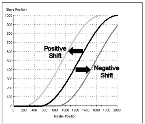
Figure 47: Illustration of the Application of Shift
