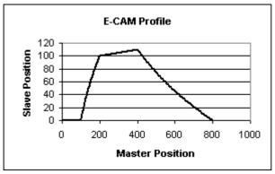
Figure 46: Sample Profile After Master Axis Scaling.
