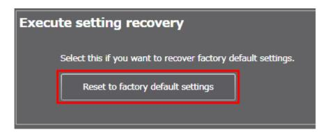
When the F3SG is in a cascade connection, select a desired sensor segment from [Target sensor] in the top right corner of the screen and click [Reset to factory default settings].
