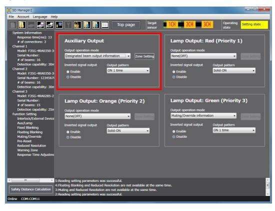
When [Designated beam output information] is selected for Auxiliary Output and each color of Lamp Output at the same time, the area configured is the same for all these outputs.
