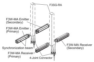
T-Shaped Configuration with 4-Joint Connector
