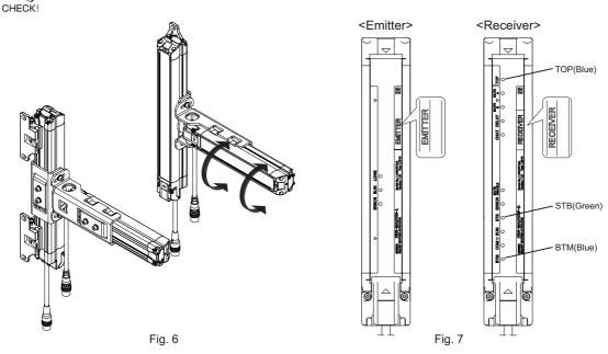
The angle of the Bracket(2) is adjustable between ±15°.
