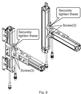
Tightening screws with a torque that considerably exceeds the recommended torque may cause failure.
