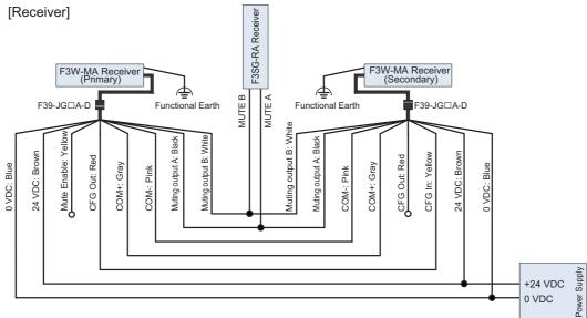
The wiring examples in later pages do not indicate functional earth. To use functional earth, wire an earth cable according to the example above. Refer to 3-4-3. Functional Earth Connection for more information.
