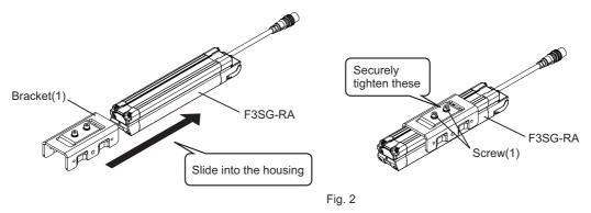
Tightening screws with a torque that considerably exceeds the recommended torque may cause failure. CHECK!
