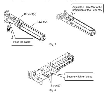
Tightening screws with a torque that considerably exceeds the recommended torque may cause failure.
