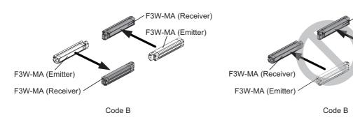
The scan code feature of the F3W-MA system allows for placement of the two systems in close proximity and in line with each other. The distinctive coding of the beams provide for unique operation of a system while in view of another system with a different scan code. Two unique codes are available on the F3W-MA.
