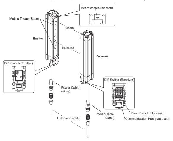
To distinguish between the emitter and receiver, find the labels attached to the front of the F3W-MA. The label on the emitter reads "EMITTER" and the label on the receiver reads "RECEIVER". CHECK!
