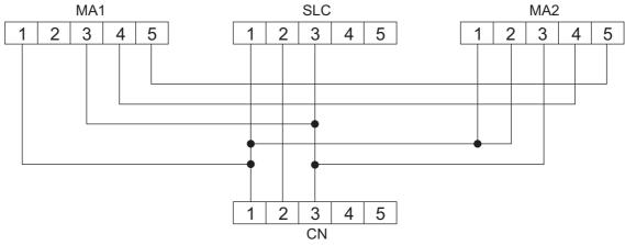
Connected to Single-Ended Cable or Double-Ended Cable for Emitter
