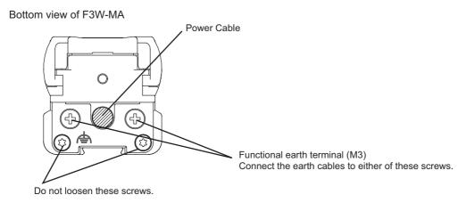
\*Select either of the terminals of the emitter and receiver according to your environment.
