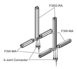
T-Shaped Configuration with 4-Joint Connector (Standard Muting)
