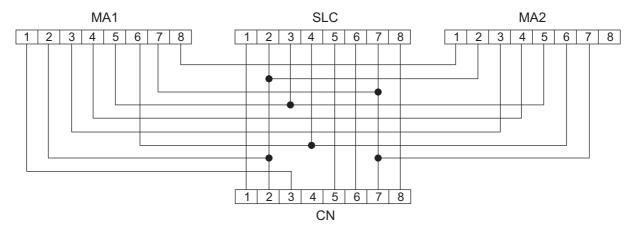
Connected to Single-Ended Cable or Double-Ended Cable for Receiver
