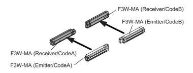
The emitter and receiver units for F3W-MA must be set to the same scan code. The scan code is selectable by the DIP Switch on the emitter and receiver units.
