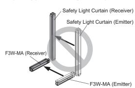
The emitter and receiver units for F3W-MA must be set to the same scan code. The scan code is selectable by the DIP Switch on the emitter and receiver units.
