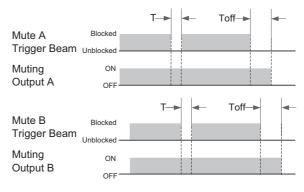
T: Time to pass through the void space Toff: Off-Delay time
