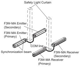
T-Shaped configuration with COM lines
