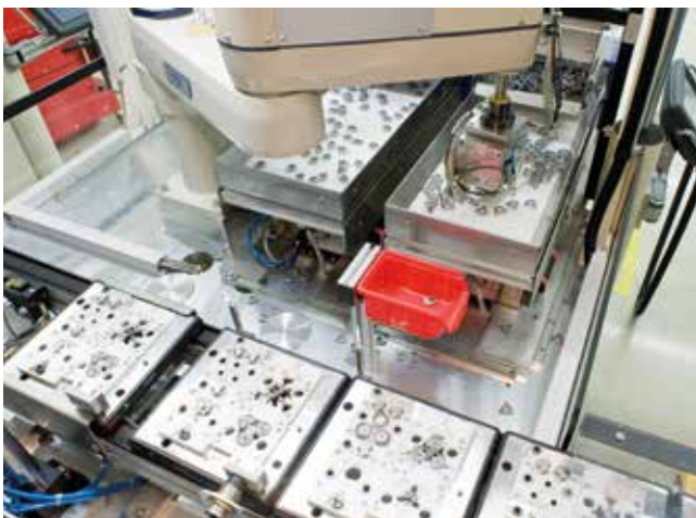
SCARA robots take over a number of challenging pick & place applications.
