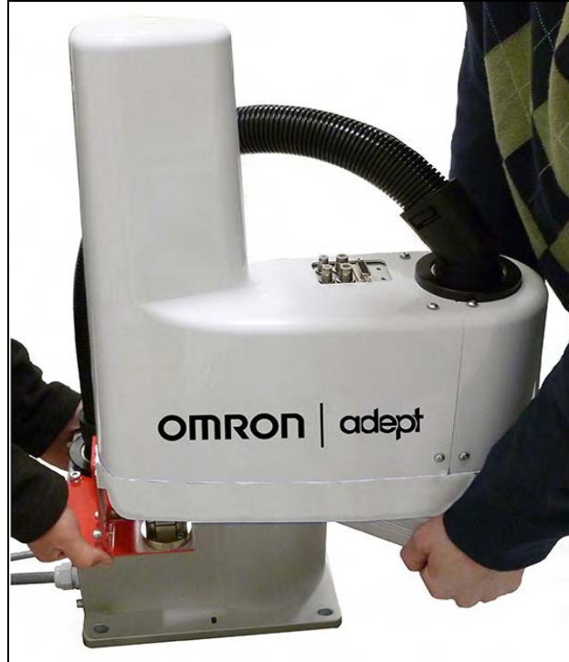
Figure 3-3. Lifting the Robot
