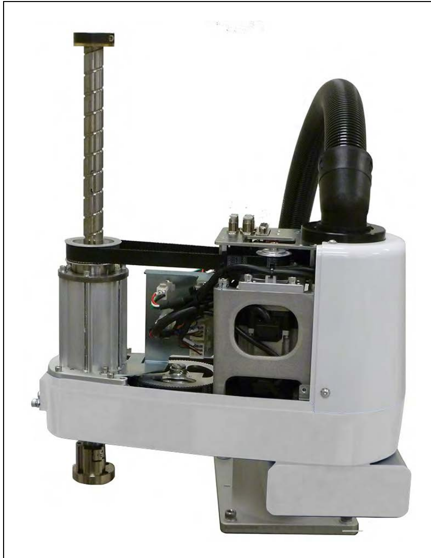
Figure 12-7. Lubrication of Joint 3 Shaft, Upper Position
