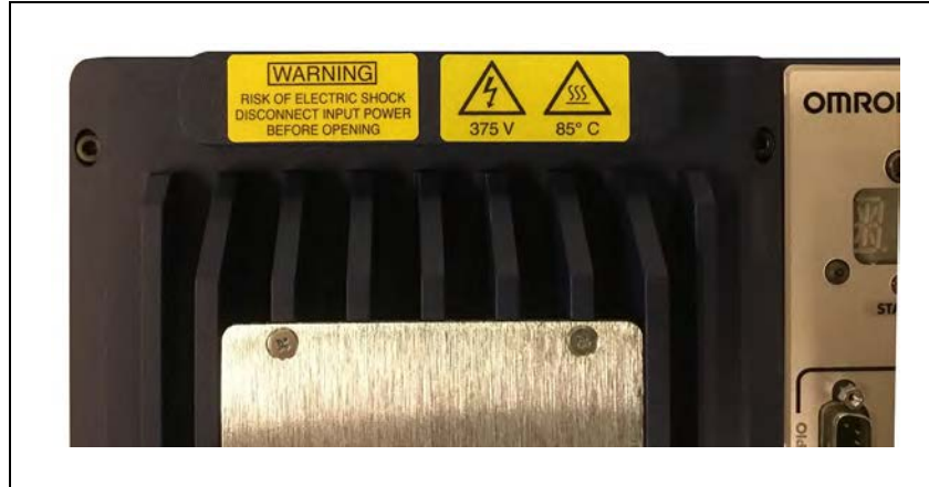
Figure 12-3. Shock and High Voltage/High Temperature Labels
