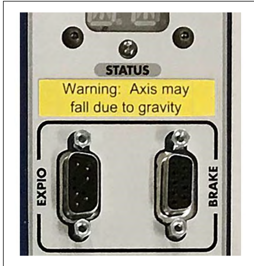
Figure 12-2. Brake-release/Gravity Warning Label
