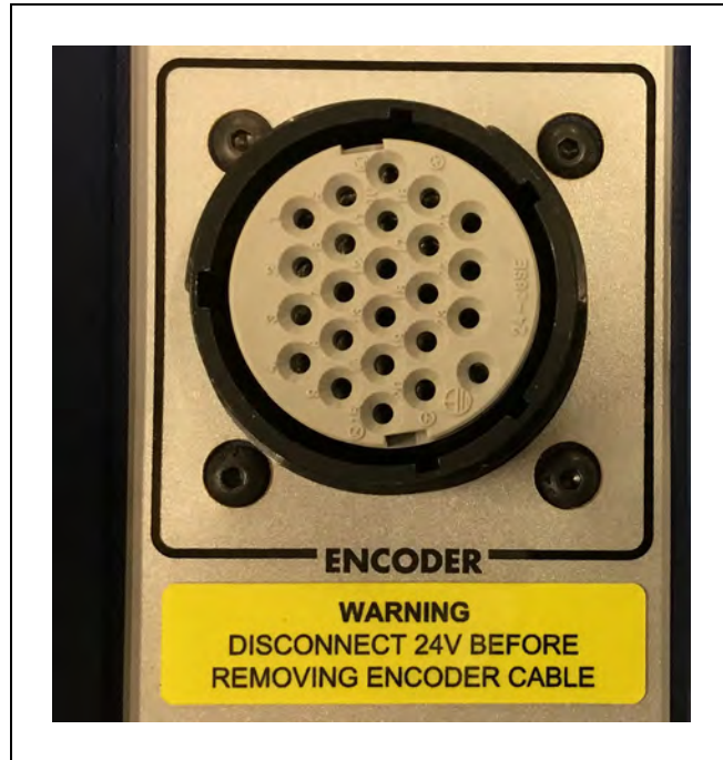
Figure 12-5. Encoder Disconnect Warning
