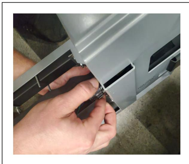
*Figure 8-38. Disconnecting the Cable*
