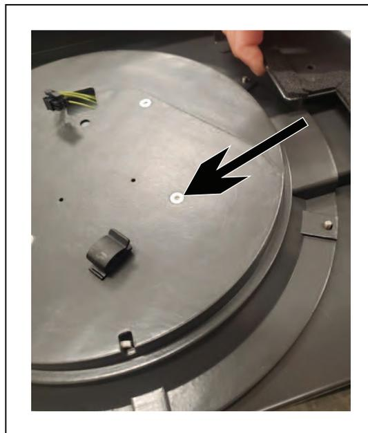
*Figure 8-30. Removing the Diffuser Plate Screws*
