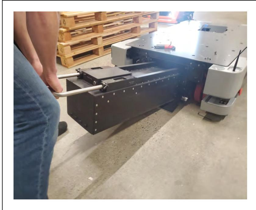
*Figure 3-59. Lifting the Battery and Pushing into the Platform*
