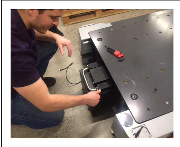
*Figure 8-24. Locking the Handle Latches*
