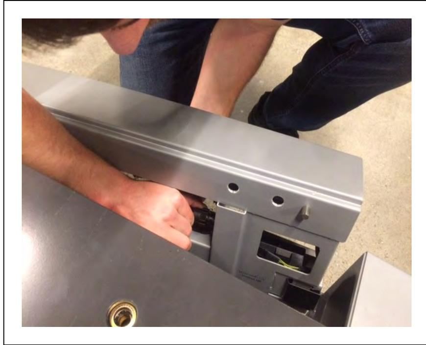
*Figure 8-34. Disconnecting Rear Skin LED Connector*
