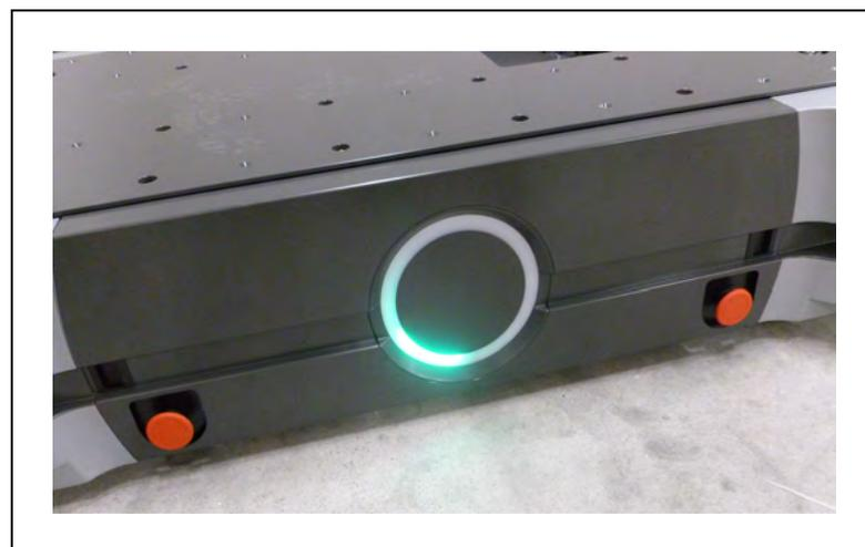
*Figure 7-9. AMR Light Disc Displaying the State of Charge (SOC)*
