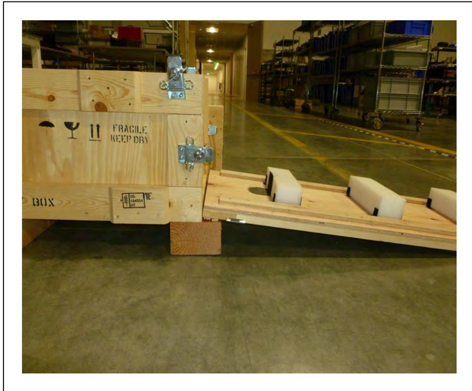
*Figure 3-31. Using the Top Cover as a Ramp*
