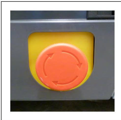
*Figure 2-4. E-Stop Button on the Platform*
