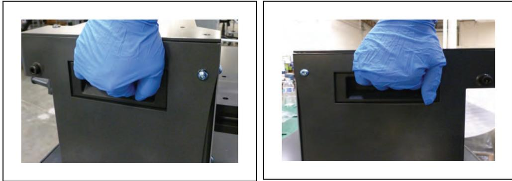
*Figure 3-45. Lifting Recesses on the Right and Left Side of the Docking Target*
