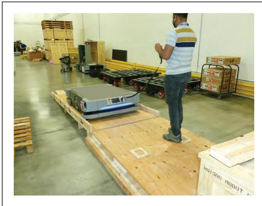
Figure 3-22. Driving the HD-1500 Down the Ramp Using the Pendant
