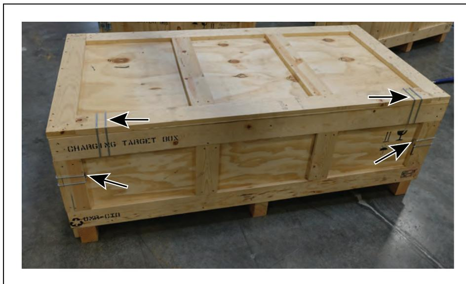
*Figure 3-39. Brackets Holding the Front Panel to the Housing Crate*
