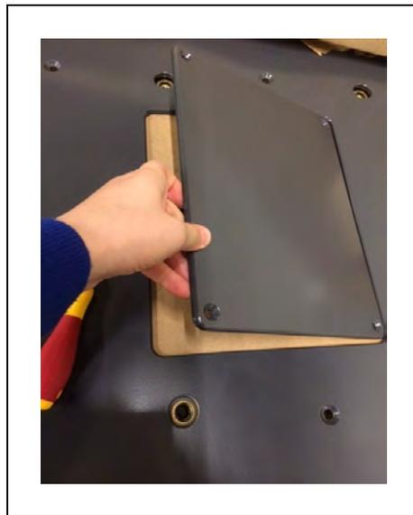
*Figure 8-60. Grabbing and Removing the Cover*
