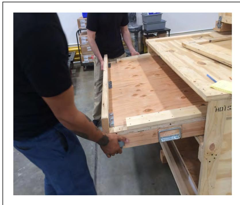
Figure 3-9. Pulling the First Ramp Out of the Crate
