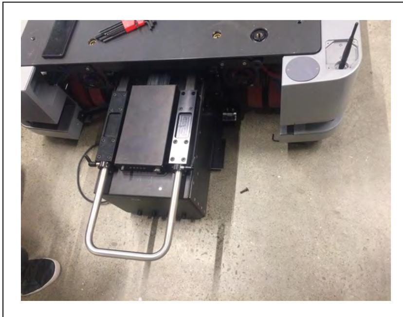
*Figure 8-17. Extending the Battery Handle Out*
