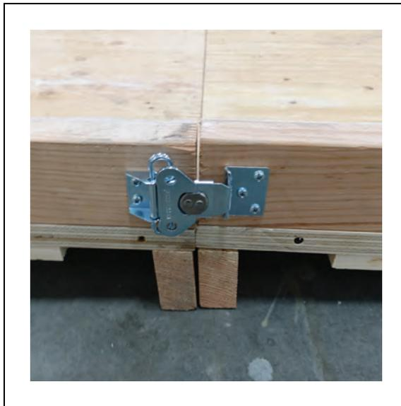
*Figure 3-17. Ramps Connected and Secured by the Locking Clips*
