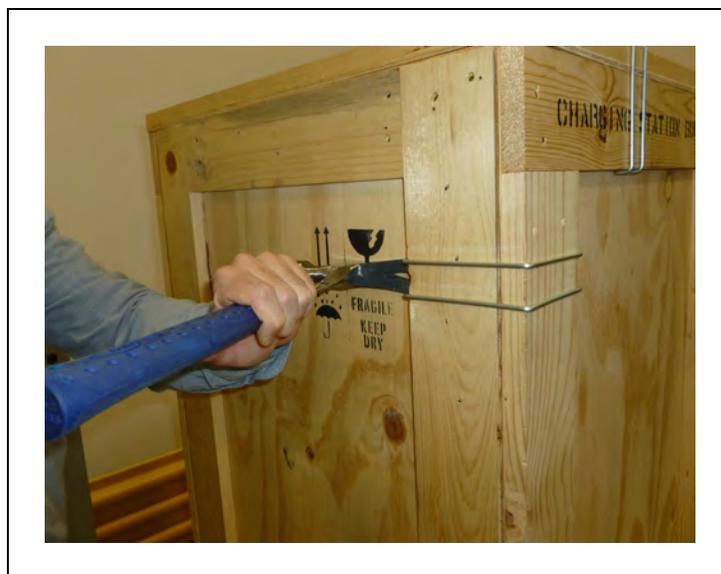
Figure 3-49. Removing the Clips
