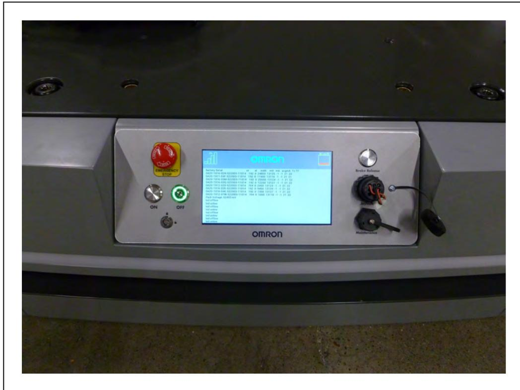
Figure 7-13. Operator Panel Installed on the HD-1500 Platform
