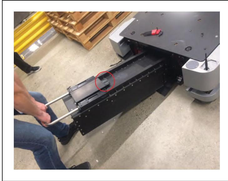
*Figure 8-18. Battery Power Connector*
