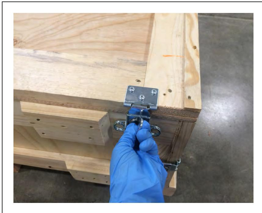
Figure 3-27. Twisting the Latch to Unlock the Top Cover
