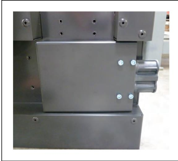
*Figure 3-72. Docking Target Power Connector Installed in Desired Orientation (Sideways)*
