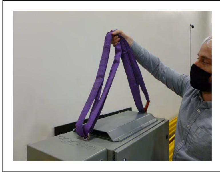
Figure 3-57. Safety-Rated Slings Attached to the Power Supply Box
