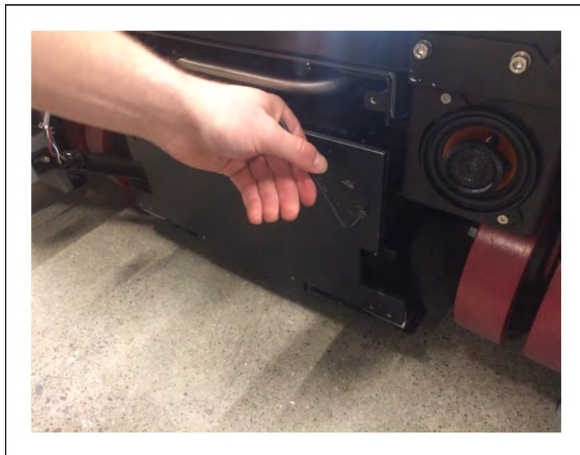
*Figure 8-13. Unscrewing the Battery Door*
