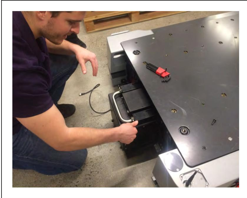
*Figure 3-61. Locking the Handle Latches*
