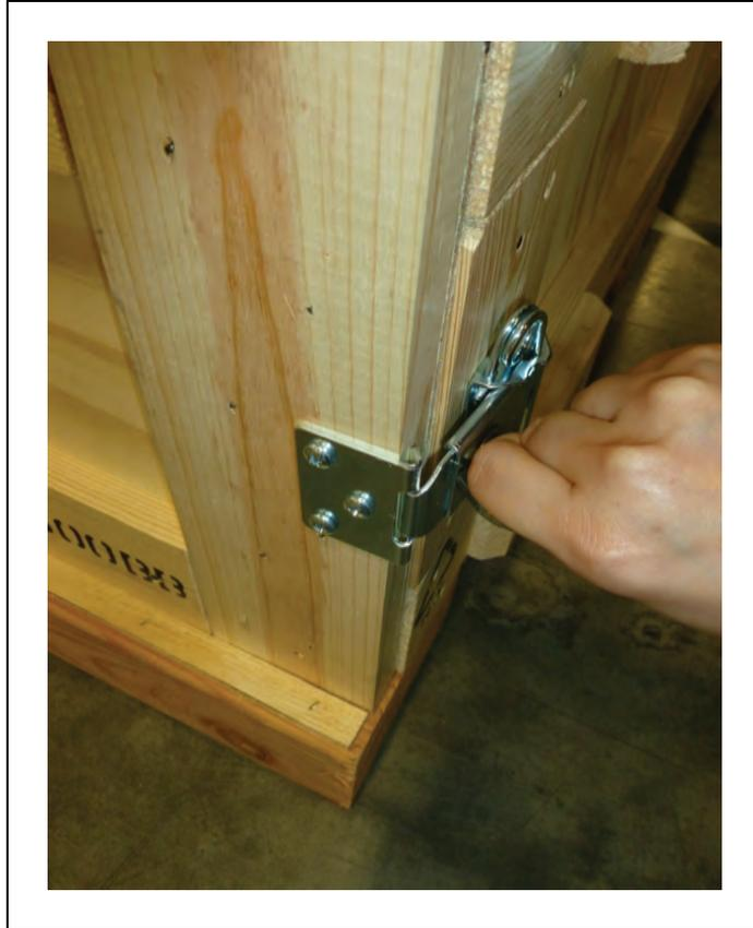
*Figure 3-29. Unlatching the Front Panel*
