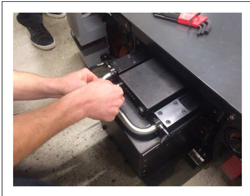
*Figure 8-15. Disconnecting the Ethernet Cable*
