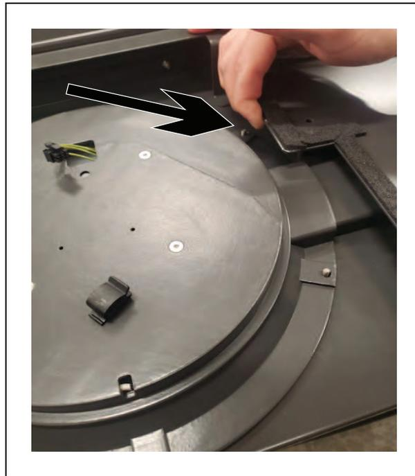
*Figure 8-29. Lifting the Electronics Bay Cover Seal to Remove the LED Mount Plate*
