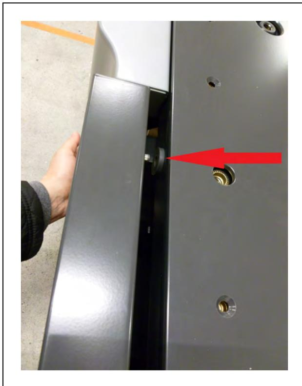
4. Install the skin on to the chassis and ensure that it latches.
