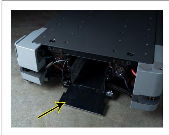
Figure 8-21. Battery Door Opens Out
