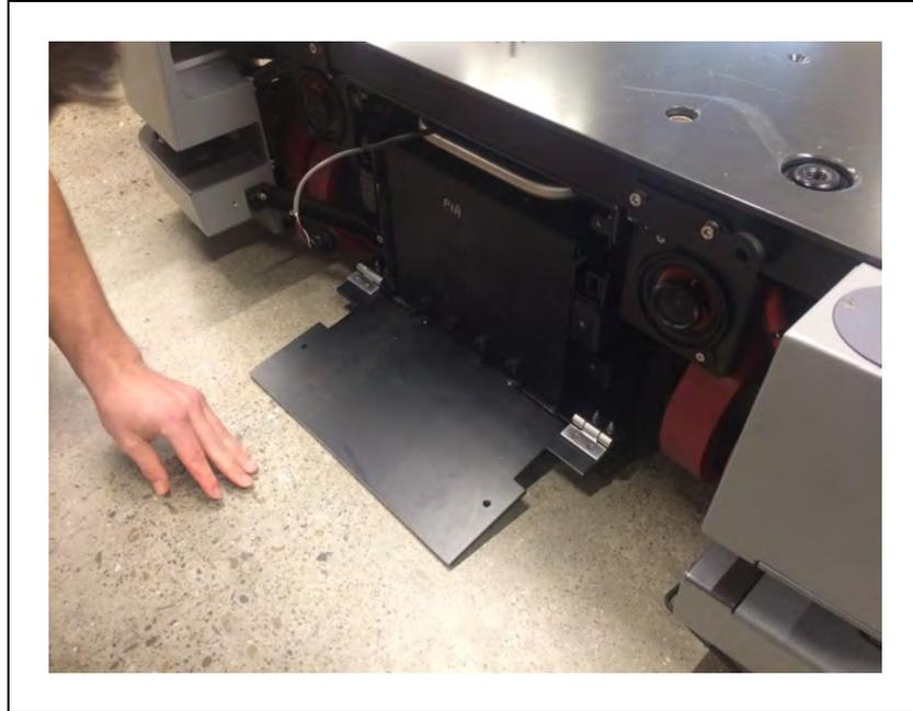
*Figure 8-14. Battery Door Opens Out, and Rests on the Floor*
