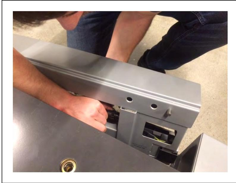
*Figure 8-47. Disconnecting the Front Light Connector*
