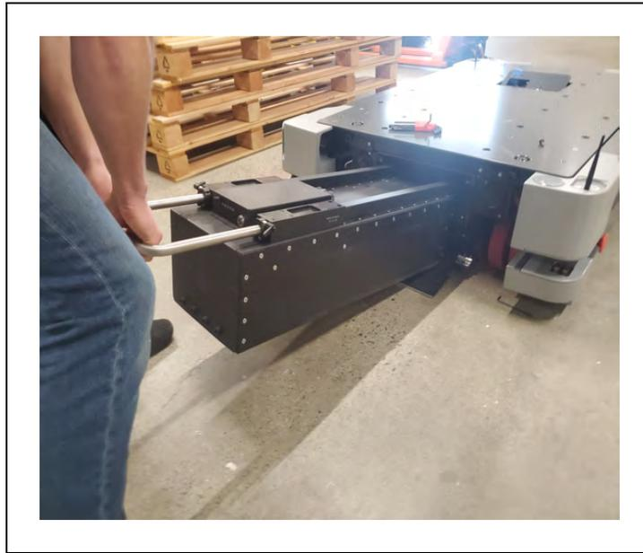
*Figure 8-22. Lifting the Battery and Pushing into the Platform*
