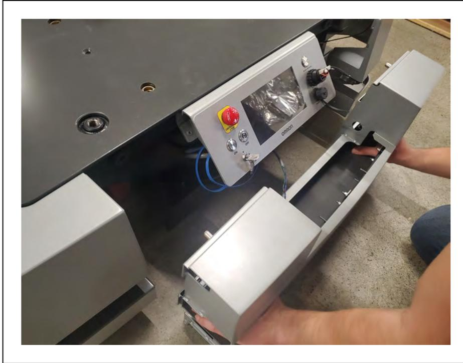
*Figure 8-52. Rear Light Cable Plugged into Its Connector*
