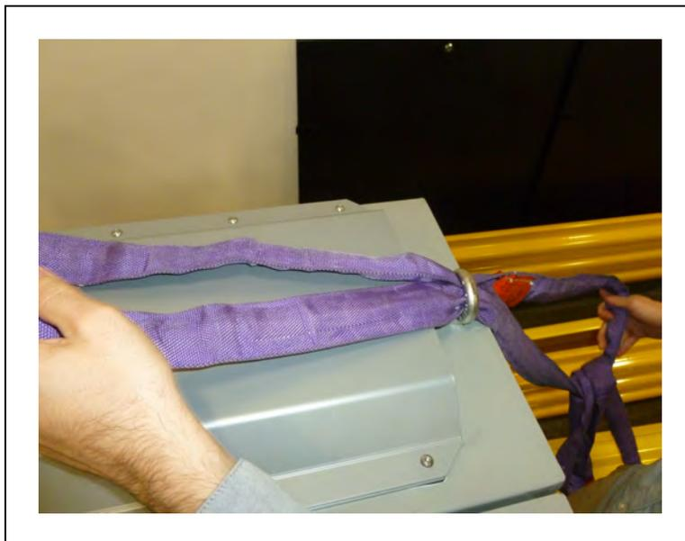
*Figure 3-56. Passing the Safety-Rated Slings Through the Eye Bolt*
