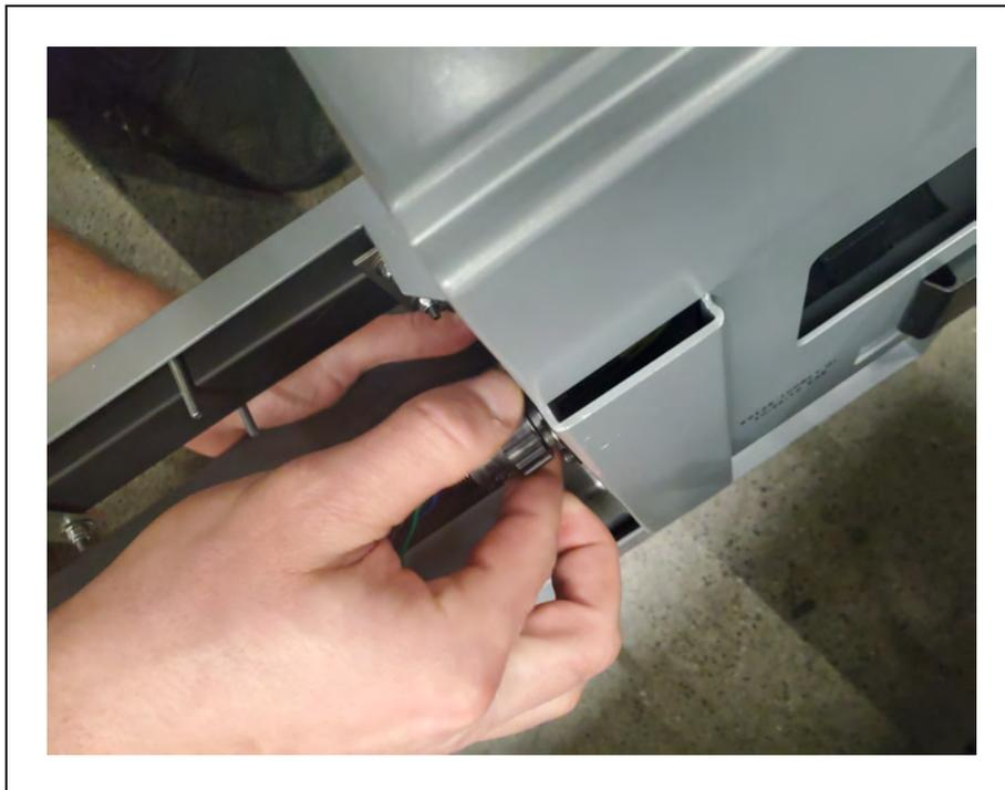
*Figure 8-53. Disconnecting the Rear Light Connector*
